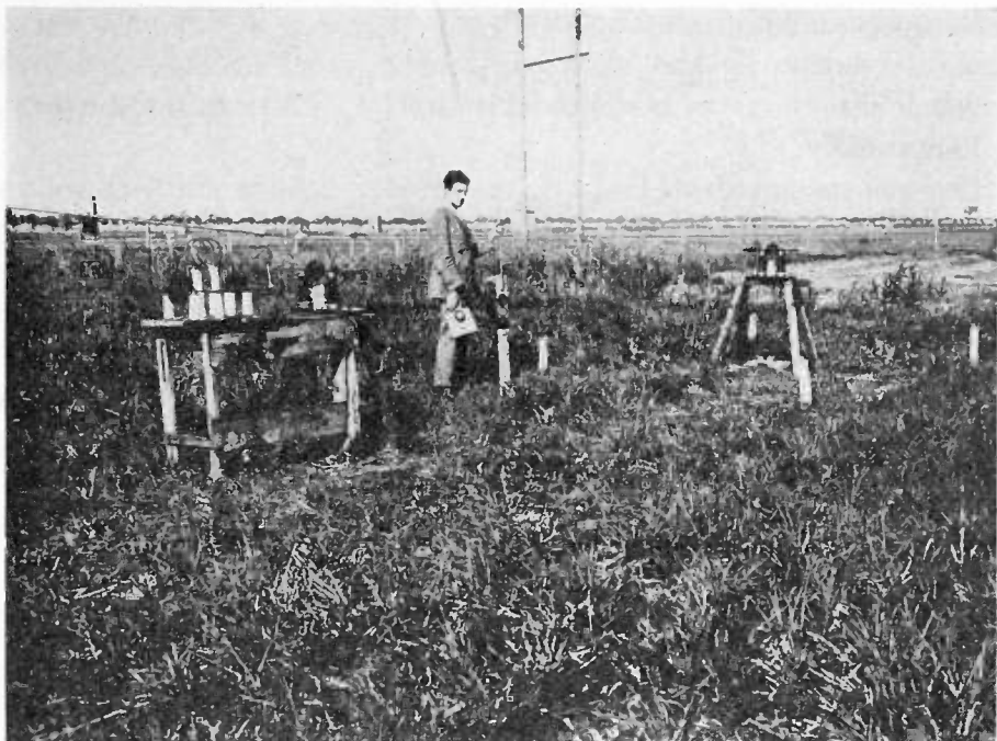
Fig. 13—Arrangements for coupling the measured line to the transmitter and for producing symmetry of the oscillation on the measured line.
