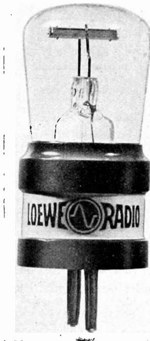
Fig. 5—Old type of luminous quartz resonator for 150 kc in metal holder.
