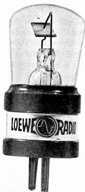
Fig. 14—A longitudinally excited luminous quartz resonator for a wavelength of about 124 meters.
