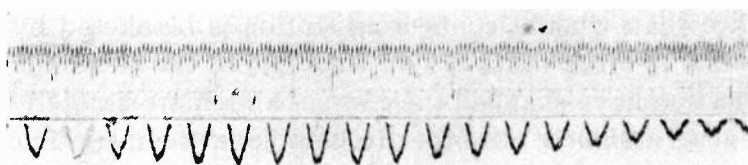
Fig. 13—Undesired modulation of a short-wave transmitter by distortion frequencies of about 500, 100, and 10 cycles. 50-cycle timing wave at bottom.
