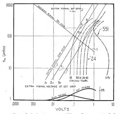
Fig. 9—Cross-talk analysis in 3-stage amplifier. Lower part of the diagram shows cross-talk contributed by 1st and 2nd stages. Volume controlled by common bias on first two tubes.
