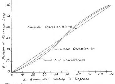
Fig. 9—Effect of the goniometer characteristic on the position of the phantom loop in space.
