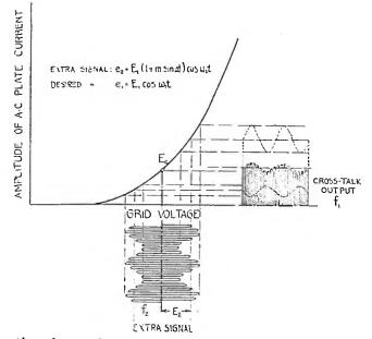
Fig. 6—Illustrating the production of Class B cross-talk. Heavy curve represents the relation between amplitude of plate current of desired-signal frequency and grid bias, with the desired signal impressed on the grid.
