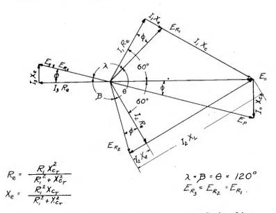
Fig. 18—Vector diagram showing phase relationships of voltages existing in Fig. 17.
