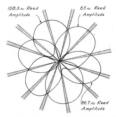
Fig. 37—Observed reed amplitude space patterns of a twelve-course radio range.
