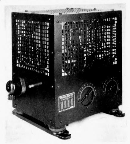
Fig. 8-Fifty-watt aircraft radio transmitter.
