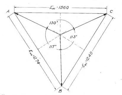
Fig. 20-Vector diagram showing method used to determine the phase relationships between each of the phases when knowing the voltages across each delta branch.
