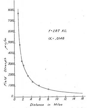
Fig. 38— Attenuation curve showing the field strength of the polydirectional radio range at different distances from the station.
