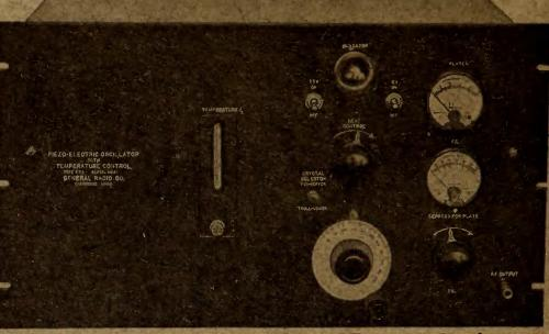
TYPE 575-A-Piezo-Electric Oscillator with Temperature Control
