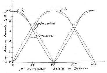
Fig. 11—Final goniometer characteristic showing deviation from theoretically perfect type.
