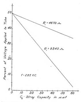
Fig. 26—Curves showing effect of stray capacity upon the per cent of total voltage  $E_p$  capable of application to the tube with different values of  $R_1$ .
