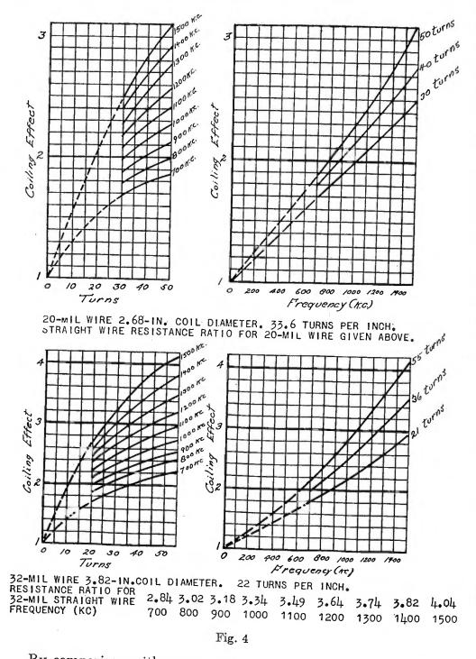
By comparison with some specific values on the curves it can be seen that the important parameters are: size of wire, number of turns, diameter of winding, and pitch of winding.
