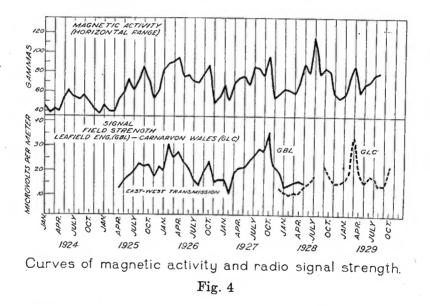
curves suggest that the connection between terrestrial magnetism and transmission may be more marked at the time of greater sun spot activity; at any rate, the correlation is poorer in 1924 than in the later years, and it appears to be decreasing in 1929 as the sun spots again begin to decrease.
