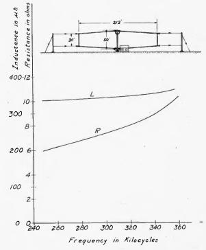
Fig. 31—Variation of antenna resistance and effective inductance with frequency.
