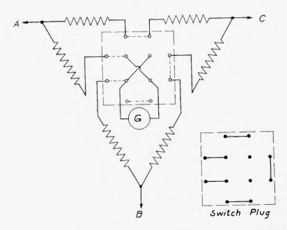
Fig. 22—Diagram showing the connections used in the instrument shown in Fig. 21.
