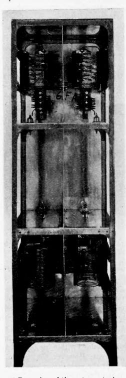
Fig. 5-Rear view of the antenna tuning unit.
