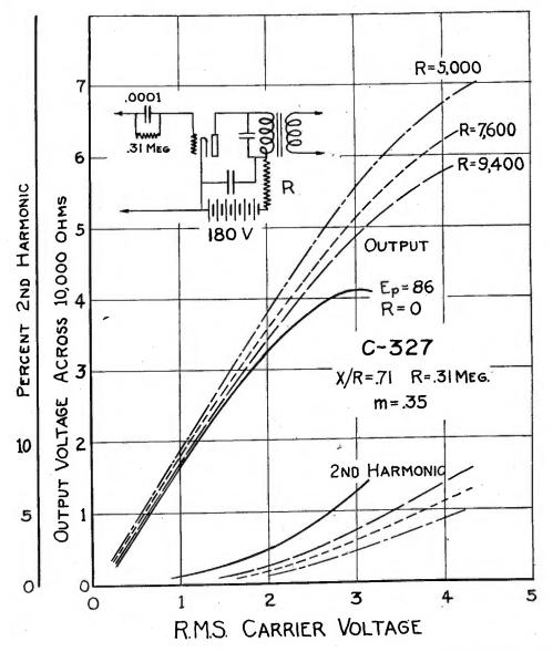
Fig. 6—Performance of grid leak power detector when operated with a high plate battery voltage that is reduced to a safe value by a series resistance, showing increased undistorted output that may be obtained with the aid of this expedient to keep the plate current to a safe magnitude.
