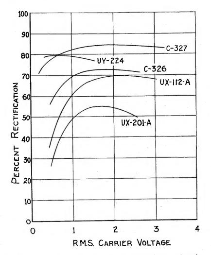
Fig. 8—Completeness of grid leak power detection as a function of signal amplitude for a number of representative tubes.
