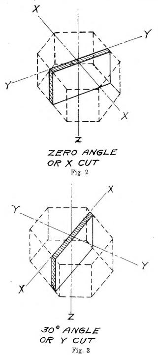
or the "Curie" cut. If they are mounted so as to yield the cut shown in Fig. 3 we have what is known as the "30-deg." or the "face parallel" cut.
