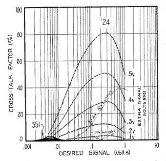
Fig. 7—Experimental curves showing cross-talk production in 24 and 551 tetrodes. Constant output maintained, corresponding to 0.001 volt desired signal at -3-volt bias.
