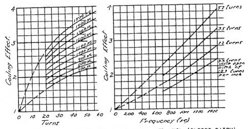
32-MIL WIRE 3.27-IN. COIL DIAMETER. 22 TURNS PER INCH (CLOSED PITCH) RESISTANCE RATIO FOR 32-MIL STRAIGHT WIRE GIVEN ABOVE.
