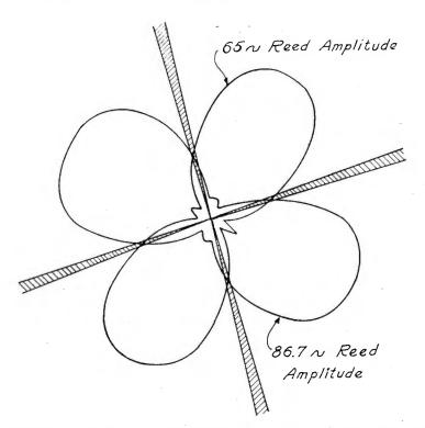
Fig. 36-Observed reed amplitude space patterns of a four-course radio range.
