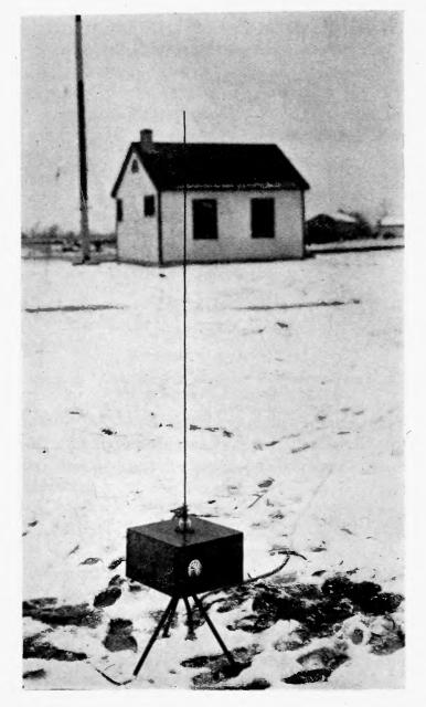
Fig. 34—Pick-up unit of course indicating device.
