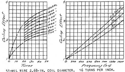
51-MIL WIRE 2.68-IN. COIL DIAMETER. 16 TURNS PER INCH. RESISTANCE RATIO FOR 51-MIL STRAIGHT WIRE GIVEN ABOVE.
