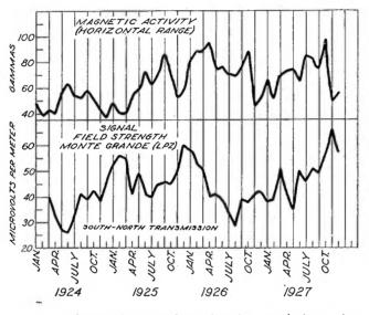
Curves of magnetic activity and radio signal strength.  ${\bf Fig.} \ {\bf 5}$
