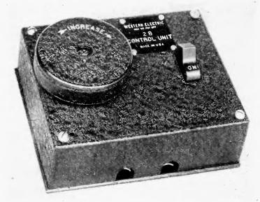
Fig. 6—Remote volume control. This includes a switch for applying power to the filament and plate circuits, and a potentiometer for controlling the shield-grid potential of the radio-frequency tubes.
