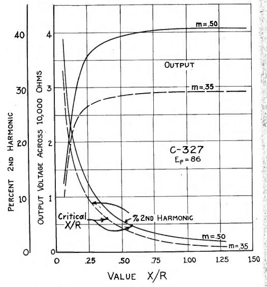
Fig. 5—Effect of X/R on sensitivity and quality, showing how both rapidly become poorer when the critical value of X/R as determined from Fig. 2 is passed.
