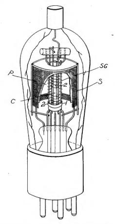
Fig. 12-Structure of tetrode of variable-mu type.
