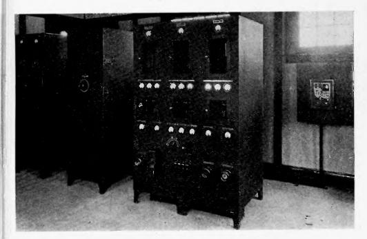
Fig. 2—General view of transmitter installation showing modulation frequency controller on the right.
