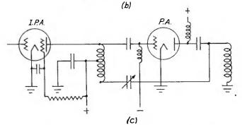
Fig. 14—(a) Schematic diagram of tuned tank coupling. (b) Schematic diagram of transformer coupling. (c) Schematic diagram of impedance coupling.
