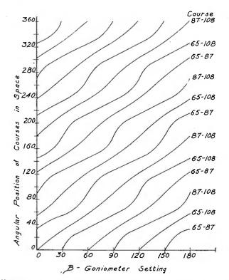
Fig. 12-Effect on course positions caused by deviation of actual goniometer from the perfect sinusoidal characteristic.
