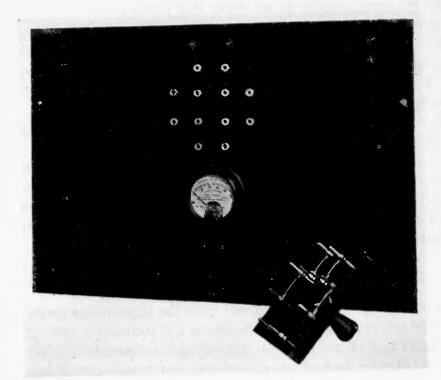
Fig. 21-View showing device used in determining the radiofrequency phase relationships.
