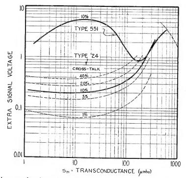
Fig. S—Diagram showing relation between tube transconductance, produced by grid bias variation, and maximum voltage of interfering signal for various percentages of cross-talk.
