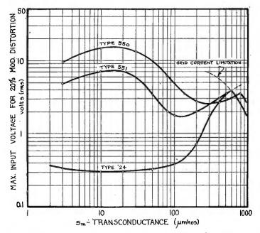
Fig. 17—Distortion limits for Types 550, 551, and 24 tubes; representing maximum input voltage which can be applied for 20 per cent modulation rise.
