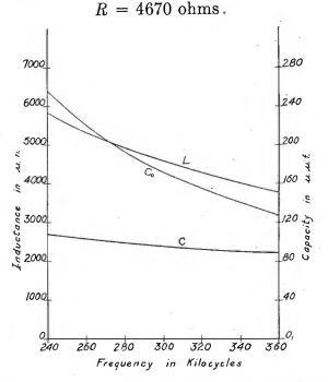
Fig. 28—Curves showing values of C, L, and  $C_0$  required for different frequencies.
