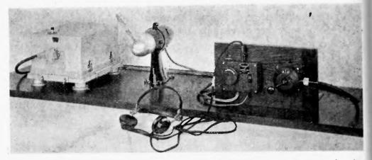
Fig: 5-Demonstration set-up of aircraft radio-receiving equipment showing type of wind driven generator.
