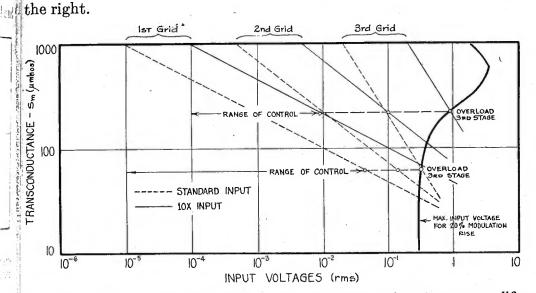
Fig. 4—Control analysis: Diagram of input voltages in a 3-stage amplifier employing 24 tetrodes; controlled by common grid bias in all stages.
