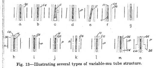
eathodes in tilted and eccentric positions; (h) and (i) show control grids of variable pitch in structures of the tetrode and triode types; (j) shows the mid-cathode control-grid gap of Fig. 11 applied to the ;riode; (k) shows a double gap and (l) a combination of gaps and variable grid pich; structure (m) is a combination of variable pitch and
