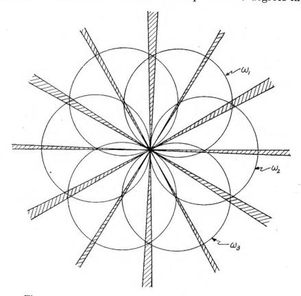
Fig. 1—Theoretical space pattern of side band fields of the triple modulation radio range.
