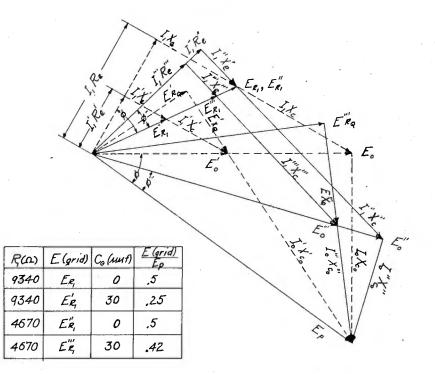
Fig. 24—Vector diagram showing the greatly reduced effect of  $C_{\mathcal{G}}$  on the available voltage supplied to the tube when utilizing a low value of shunt resistance.
