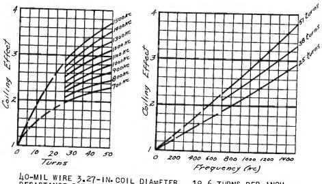
40-MIL WIRE 3.27-IN. COIL DIAMETER. 19.6 TURNS PER INCH. RESISTANCE RATIO FOR 40-MIL STRAIGHT WIRE GIVEN ABOVE. Fig. 6
