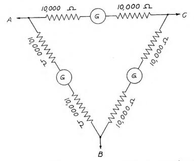
Fig. 19—Diagram showing delta arrangement used to determine the radiofrequency time phase relationship between each of the phases.
