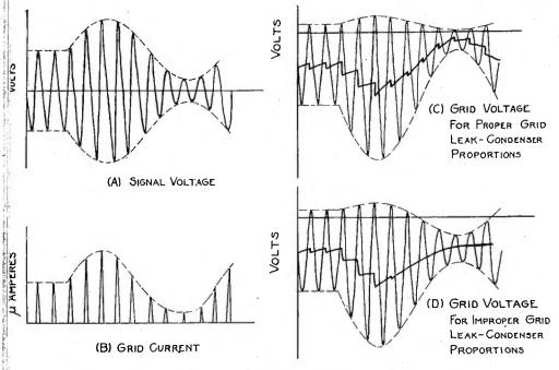
Fig. 1—Details involved in the detection of large signals by means of grid leak and grid condenser.
