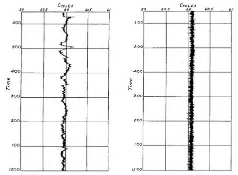
Fig. 7-(a) Frequency variation of commercial power network manually controlled. (b) Frequency variation of sixty cycles obtained from the inverted rotary converter when using frequency controller.
