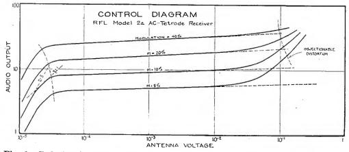
Fig. 3—Relation between audio output and antenna voltage in a receiver employing automatic volume control, exhibiting modulation rise and distortion at high input voltages.
