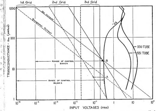
Fig. 5—Control analysis for graduated bias control; stage 3 uncontrolled; stages 1 and 2 controlled by common bias. Other conditions identical with Fig. 4.
