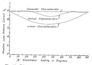
Fig. 10-Effect of the goniometer characteristic on the current in the phantom loop.
