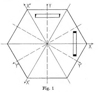
cut. Owing to the evident ambiguity in the use of any of the last three, the term "Curie cut" is preferable. However, a still more concise term would be the "X-cut," denoting a plate the normal to whose face, and hence for which the applied electric field, is parallel to an X-axis.
