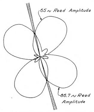
Fig. 35-Observed reed amplitude space patterns of a two-course radio range.
