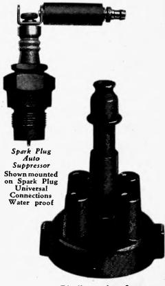
Distributor Auto Suppressor Shown mounted on distributor cap. Fully insulated, no metal parts exposed, rigid mounting.
