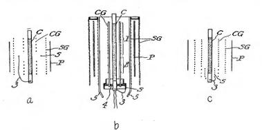
Fig. 14—Several types of variable-mu structure.
