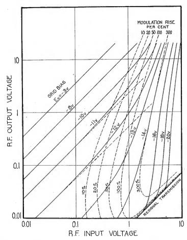
Fig. 2—Input-output voltage diagram for a single tuned r-f amplifier stage employing type 24 tetrode ( $E_b = 180 \text{ v}$ ;  $E_d = 90 \text{ v}$ ). The dotted lines are contours of constant modulation rise.
