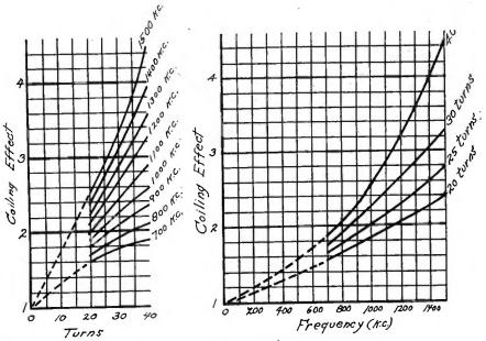
20-MIL WIRE3.82-IN. COIL DIAMETER.33.6 TURNS PER INCH.RESISTANCE RATIO FOR1.831.982.12.22.32.472.552.6420-MIL STRAIGHT WIRE700800900100011001200130014001500
