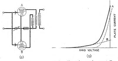
Fig. 11-Method of decreasing distortion and cross-talk.
