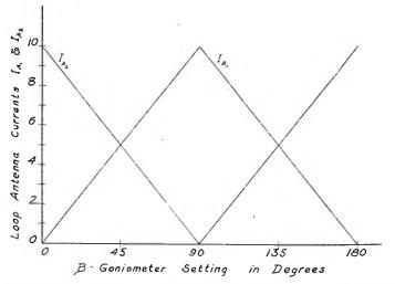
Fig. 8—Linear characteristics of a theoretical goniometer, showing the relation between goniometer setting and antenna current.
