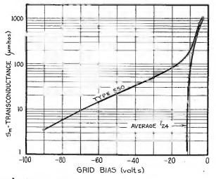
Fig.16-Transconductance-grid voltage characteristic of Types 550 and 24 tubes.
