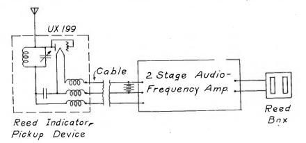
Fig. 33-Schematic diagram of course indicating device.
