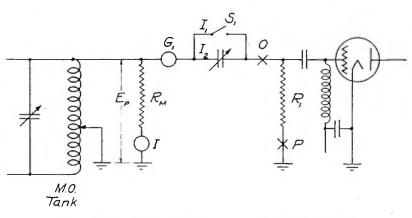
Fig. 29—Schematic diagram showing methods used in determining the voltage ratio.
