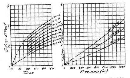
32-MIL WIRE 2.68-IN. COIL DIAMETER. 22 TURNS PER INCH. RESISTANCE RATIO FOR 32-MIL STRAIGHT WIRE GIVEN ABOVE.
