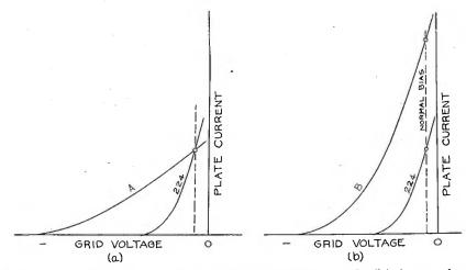
Fig. 10—Showing (a) decreasing transconductance and (b) increasing plate current accompaning attempts to decrease distortion by decreasing the mu-factor.
