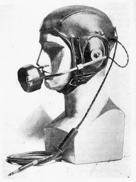
Fig. 10—Pilot's headset with close-talking microphone and phonette-type earpieces attached. This arrangement leaves both hands free for the controls.
