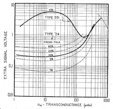
Fig. 8-Diagram showing relation between tube transconductance, produced by grid bias variation, and maximum voltage of interfering signal for various percentages of cross-talk.
