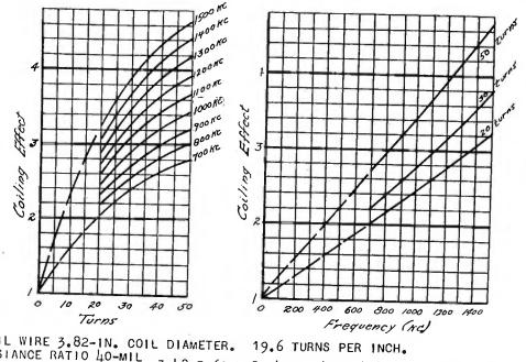
40-MIL WIRE 3.82-IN. COIL DIAMETER.19.6 TURNS PER INCH.RESISIANCE RATIO 40-MIL<br/>STRAIGHT WIRE3.48 3.69 3.82 4.11 4.33 4.49 4.66 4.82 4.97FREQUENCY (KC)700 800 900 1000 1100 1200 1300 1400 1500
