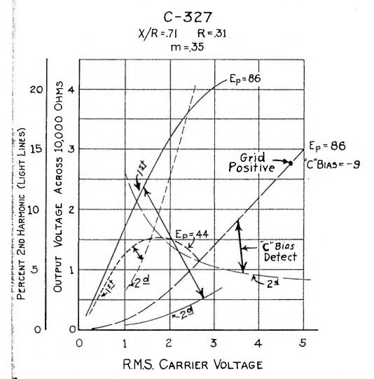
Fig. 4—Performance of grid leak and "C" bias power detectors under favorable conditions. The solid and dotted lines are for grid leak detection, while the dash line applies to plate rectification.
