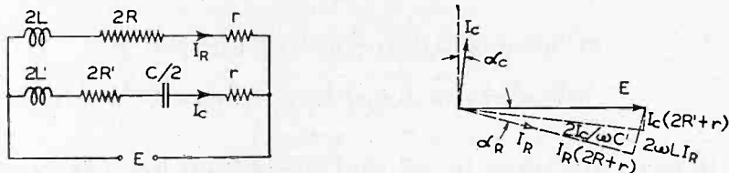
Fig. 5— Simplified circuit of potentiometer. Fig. 6— Vector diagram of simplified circuit.
