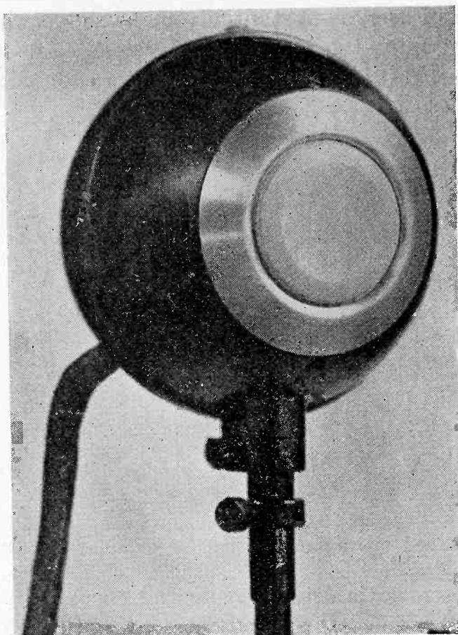
Fig. 5—Assembled microphone and standard spherical mounting.
