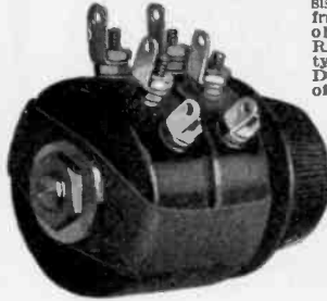
No. 2880-2880. Bakelite shell composition element only. Resistance range from 5,000 ohms to 1 megohm. All curves. Potentiometer or rheostat types. Units insulated from each other. Diameter, 1 1/2 in. Depth of shell, 1 1/8 in.
