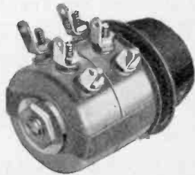
No. 2880-2880. Bakelite shell composition element only. Resistance range from 5,000 ohms to 1 megohm. All curves. Potentiometer or rheostat types. Units insulated from each other. Diameter, 1 1/2 in. Depth of shell, 1 1/8 in.
