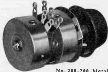
No. 200-200. Metal shell type wire wound resistors with resistances from 5 ohms to 10,000 ohms. Split windings. Rheostat or potentiometer types. Units insulated. Diameter, 1 7/16 in. Depth of shell, 1 1/2 in.
