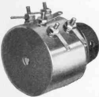
No. 890. Double depth metal shell unit in rheostat or potentiometer type. Rotors in same electrical connection. Composition elements, 5,000 ohms to 1 megohm in each unit. Diameter, 1 7/8 in. Depth of shell, 1 3/16 in.
