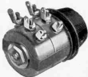
No. 2880-2880. Bakelite shell composition element only. Resistance range from 5,000 ohms to 1 megohm. All curves. Potentiometer or rheostat types. Units insulated from each other. Diameter, 1 1/2 in. Depth of shell, 1 1/8 in.
