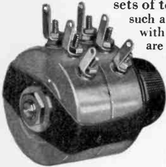
No. 280-280. Combination metal shell wire wound and composition elements. Wire wound up to 15,000 ohms. Composition, 5,000 1 megohm. Rheostat or potentiometer type in either unit. Units insulated from each other. Diameter, 1 11/16 in. Depth of shell, 1 3/8 in.
