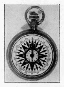
Fig. 3-Stop Watch Fitted with Special "Compass-Card" Dial for Use in Taking Bearings from a Rotating Beacon.
