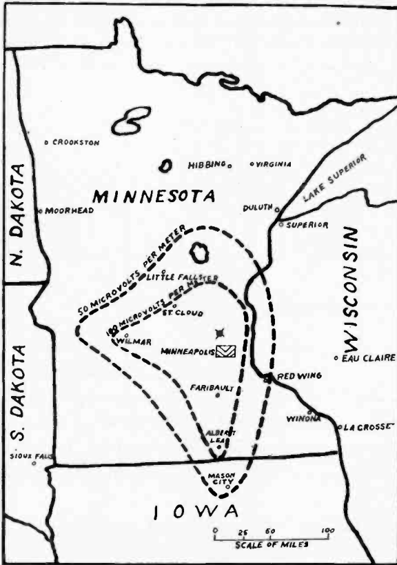
Fig. 1—Daylight Distribution of Radio Field from WCCO, 720 kc, 5000 watts.
