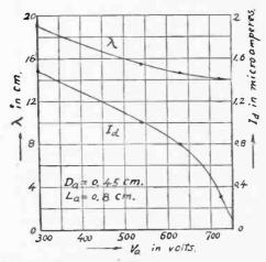
Fig. 28-Variation of Wavelength with Voltage.
