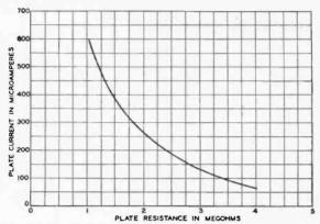
Fig. 9-Plate-Current, Plate-Resistance Characteristics of CX-322.
