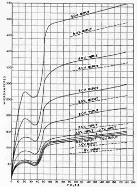
Fig. 6—Plate Current—Plate Voltage Characteristics of CX-322. Variable Input Voltages.  $Ec_1 = -7.5$ ;  $Ec_2 = +4.5$
