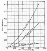
Fig. 4—Characteristics of Tube B with 150 Volts on Plate, 50 Volts on Outer Grid, and 16.5 Amperes Filament.
