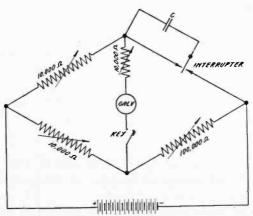
Fig. 9-Maxwell Bridge Circuit.
