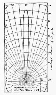
Fig. 13-Beam Radiation from a Radiator Utilizing a Wave Canal.
