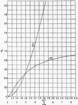
Fig. 13—Space Charge for Concentric Cylindrical Anode and Cathode of Infinite Length.
