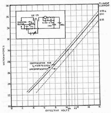
Fig. 3-Compensated Electron Tube Voltmeter; Plate Current Method.
