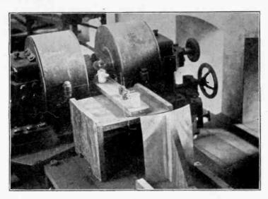
Fig. 27-Apparatus Set-up for the Shortest Waves Obtained (14-15 cm.).
