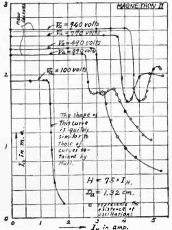
Fig. 25—Variation of Anode Current with Strength of Magnetic Field.
