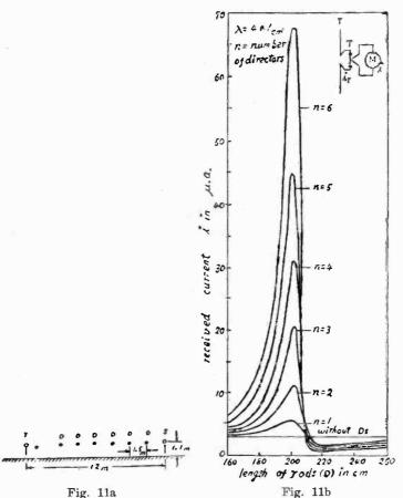
The Effect of Varying Number and Length of Directors in Wave Canals on Received Current.
