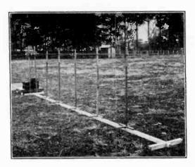
Fig. 19-Projector Horizontally Polarized Wave; 260 cm.
