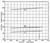
Fig. 4-Mutual Conductance-Plate Voltage Characteristics of CX-322.
