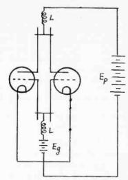
Fig. 1-Circuit Diagram of Oscillator; 60-200 cm.
