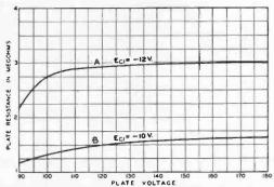
Fig. 5—Plate Resistance—Plate Voltage Characteristics of CX-322.  $A = Ec_1 = 12.0, Ec_2 = +67.5$  $B = Ec_1 = 10.0, Ec_2 = +67.5$
