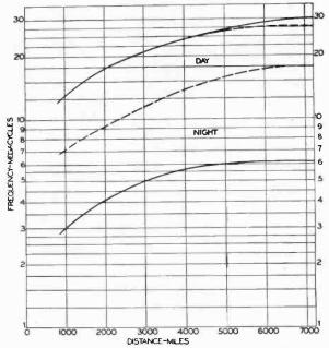
Fig. 1—Approximate Relation of Optimum Frequency to Distance in Short Wave Radio Transmission. 1½ to 30 megacycles, 0 to 7000 miles.
