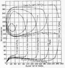
Fig. 3—Characteristics of Tube B with 250 Volts on Inner Grid and 15 Amperes Filament. Principal Dimensions: plate, 3½ in. long by 1½ in. in diam.; filament, 6½ in. of 18 mil. wire (V-shaped); outer grid 1¼ in. in diam. 13 turns per inch of 10 mil. wire; inner grid, ¾ in. in diam. 13 turns per inch of 10 mil. wire.
