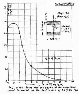
Fig. 26-Variation of Oscillation Intensity with Tube Position in Magnetic Field.
