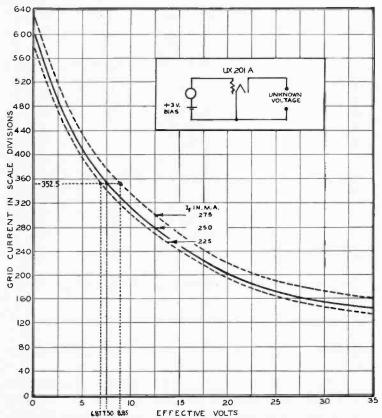
Fig. 1-Uncompensated Electron Tube Voltmeter; Grid Current Method.
