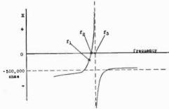
Fig. 6-Reactance of Resonator N2
