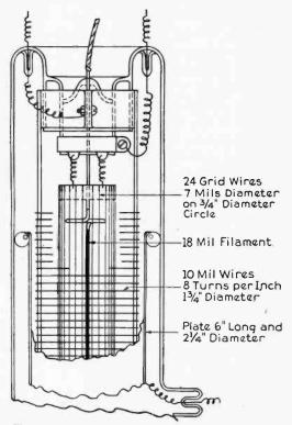
Fig. 5-Tube C-Four-Element Vacuum Tube.
