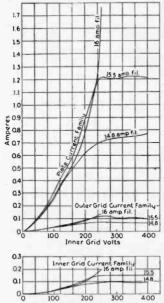
Fig. 7—Characteristics of Tube C with 150 Volts on Plate and 75 Volts on Outer Grid.
