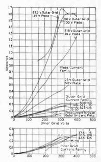
Fig. 9-Characteristics of Tube C with 16.0 Amperes Filament Current.
