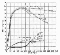
Fig. 2—Characteristics of Tube A with 125 Volts on Plate. E. is the Anode or Outer Grid Potential.
