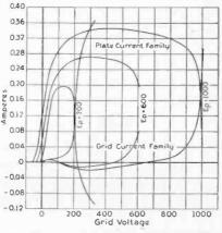
Fig. 1—Characteristics of a 250-Watt Pliotron.
