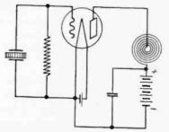
Fig. 2—Circuit Used in Navy Standard Oscillator to Develop Harmonics of Crystal Frequency
