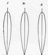
Fig. 36-Polar Curves. 1-Calculation; 2-Horizontal Observed; 3-Vertical Observed.
