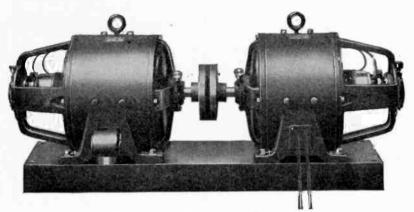
Type P Two Unit Motor Generator
