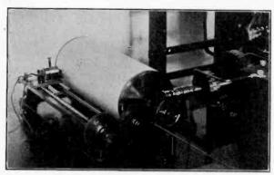
Fig. 8—Chronograph Drum, with Paper Mounted for Calibration Record. Recording Relay at Left, on Carriage.
