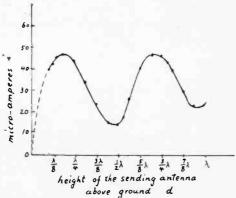
Fig. 18-The Effect of Height of Sending Antenna on Receiver Current.
