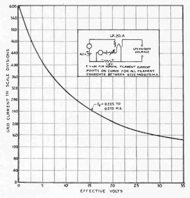
Fig. 2-Compensated Electron Tube Voltmeter; Frid Current Method.
