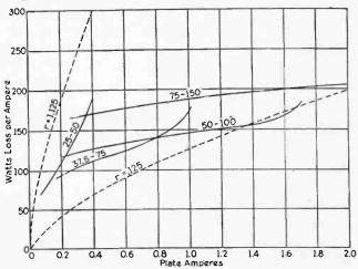
Fig. 14—Loss in Tube C in Watts per Ampere. Solid Curves Are for Tube C. The Figures Indicate Outer Grid and Plate Potentials. Dotted Curves Are for Kenotrons of Radii Indicated.
