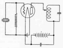
Fig. 1—Tuned Plate Type of Crystal Oscillator Circuit, Having a Low L/C Ratio.
