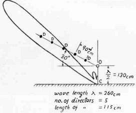
Fig. 22-Polar Diagram with Wave Canal at 30 deg. to Surface of the Earth.
