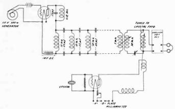
Fig. 10-Crystal Calibrating Circuit.
