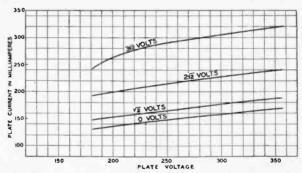
Fig. 8—Plate-Current, Plate-Voltage Characteristics of CX-322. R=400,000 ohms
