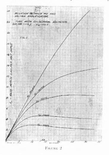
are small. This condition usually exists in all but the last tube of an amplifier, but in this tube the amplitudes must be large, since the power supplied to the loud speaker is often considerable. It then becomes necessary to determine the output characteristics of the tube feeding the loud speaker, and in particular it is
