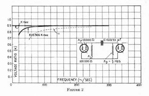
$f_o$ , say 50 cycles per second, a certain fraction, k, of the maximum voltage ratio possible with the given combination of resistances.
