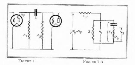
voltage of the coupling device and is impressed on the input of the second tube.  $V_p$  is the voltage input to the coupling device and equal to the voltage impressed on the input of the first tube multiplied by the voltage amplification constant of that tube or  $\mu e_p$ . The solution of Figure 1A follows:
