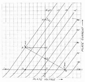
FIGURE 7--- Tube Characteristics for Showing Conditions for Maximum Understorled Output
