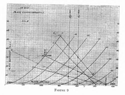
family of plate voltage—plate current curves for the UX-210 Radiotron which will be used for these illustrations. This tube has been designed for use as an oscillator or as an amplifier for plate voltages not exceeding 400 volts. As an oscillator the tube is rated at 7.5 watts output, and the safe plate power dissipation is 12 to 15 watts, depending somewhat on the conditions of use.
