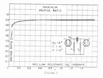
ratio is 90 per cent of the maximum attainable voltage ratio at the output of the amplifier. If there are two identical stages in the amplifier the value of k per stage will be  $\sqrt{.90}$  (or 0.949); if there are three identical stages the value of k per stage will be  $\sqrt[3]{.90}$  (or 0.966).
