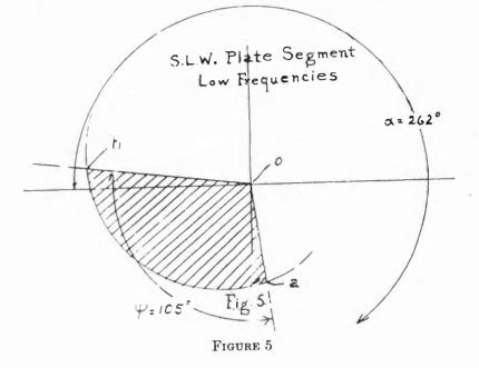
is the actual total plate rotation, g is the ratio of maximum<sup>5</sup> to minimum wave length and a is the angle of the shortest polar radius vector used in Figure 3, corresponding to the shortest radio edge (in the S.L.F. plate it is the *longer* radial edge) of the condenser plate.
