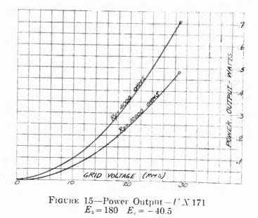
volt squared input—and the square of the r.m.s. grid voltage for  $P_{max}$  will not always check exactly the figure given for  $P_{max}$ itself, as this latter was obtained in every case by graphical methods.
