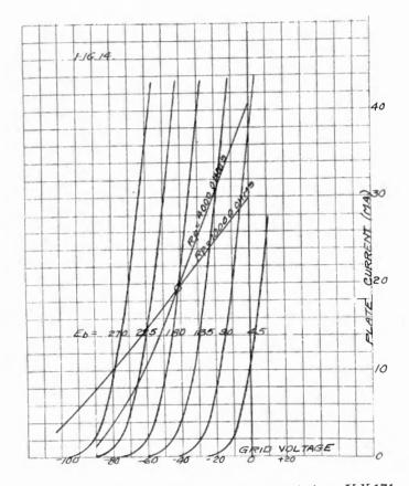
FIGURE 14-Static and Dynamic Characteristics-UX 171
