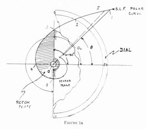
this angle is  $\theta$  and gives  $C_o$  or a zero capacitance, corresponding to stray capacitances which make up the polar area to infinity beyond his  $\theta = 0$ , which is really 270 deg. or  $3\pi/2$ . This fictitious area for outside capacitances  $C_o$  is  $A_o$ .
