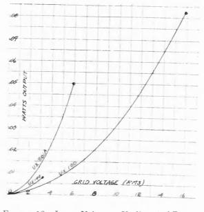
FIGURE 13—Input Voltage—Undistorted Power Output—Load Resistance 20,000 Ohms  $UX 120 - E_5 = 135$ ,  $E_c = -22.5$  $UX 199 - E_b = 90$ ,  $E_c = -4.5$  $UX 201.4 - E_b = 135$ ,  $E_c = -9.0$
