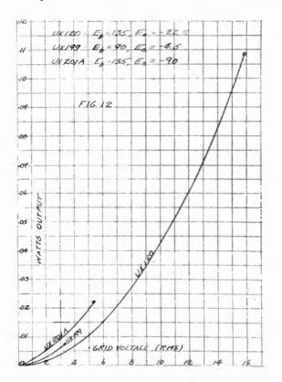
FIGURE 12—Input Voltage—Undistorted Power Output—Load Resistance 10,000 Ohms
