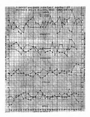
The degree of temperature—signal relationship may be judged from the accompanying curves for the year 1924. In the curve of monthly averages for the year, the average daylight signal intensity of the two stations corrected for antenna current changes is shown in millivolts per meter with the corresponding curve of 100/temp. (F.). The curves of daily averages for each month represent the plus and minus deviations of the signal intensity and of the temperature from the monthly means.
