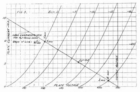
FIGURE 5-Tube and Load Characteristics
