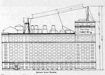
FIGURE 4-Plan-Elevation of the Transmitting Antenna
