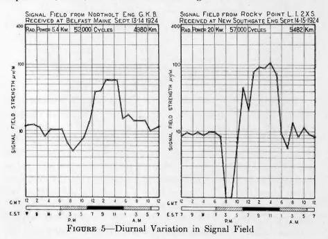
upper curves are for similar averages of measurements made on the lower frequencies. These curves show clearly that the range of the diurnal fluctuation is less for the lower frequencies. This is because of the lesser daylight absorption.
