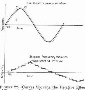
FIGURE 22—Curves Showing the Relative Effect of Transmission Time Lag in Sinusoidal and Stepby-step Methods of Frequency Variations
