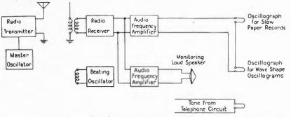
FIGURE 6-Diagram of System Used for Single Frequency Tests
