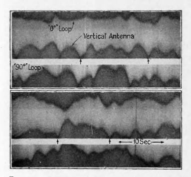
FIGURE 36—Single Frequency Fading Record from Vertical Antenna and Two-Loop Antenna Crossed at Right Angles
