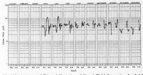
Monthly Averages of Diurnal Variation of Signal Field Strength. Leafield England. (GBL) Measured at Belfast, Maine. Corrected to 300 Amperes Antenna Current 24,050 Cycles
