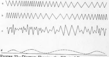
FIGURE 23—Diagram Showing the Effect of Frequency Modulation
