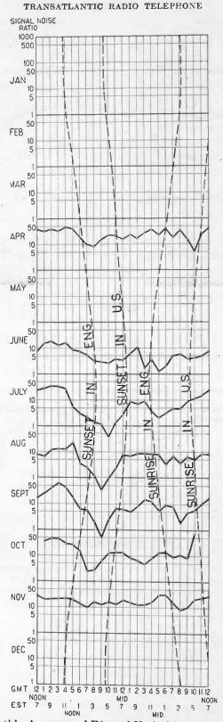
FIGURE 27—Monthly Averages of Diurnal Variation in Signal-to-Noise Ratio. Northolt, England. (GKB) Received at Belfast, Maine. Corrected to 20,8 kw. Radiated. 4,980 km. 52,000 Cycles. 1924
