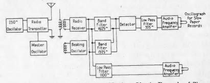
FIGURE 49—Diagram of System Used to Obtain Records of Transmission with Carrier and One Side Band and Carrier and Both Side-Bands
