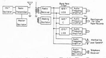
FIGURE 11—Diagram of System Used for Three-Frequency Tests
