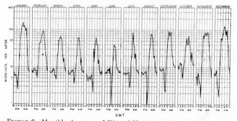
FIGURE 8—Monthly Averages of Diurnal Variation in Signal Field. Rocky Point, L. I. (2XS) To New Southgate, England. 57,000 Cycles—Antenna Current, 300 Amperes—5,480 Km. 1923—1924
