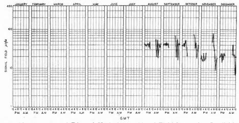
Monthly Averages of Diurnal Variation of Signal Field Strength. Leafield, England (GBL) Measured at Riverhead, L. I. Corrected to 300 Amperes Antenna Current.
