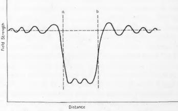
FIGURE 32—Theoretical Cross-Section of Radio Shadow and Associated Wave Interference Pattern
