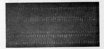
FIGURE 9-Wave Form of Beat Note Signal for Single-Frequency Test. Center Trace Signal from Vertical Antenna, Upper and Lower Traces Signals from Loop Antenna Receivers
