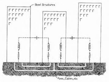
FIGURE 27—Idealized Picture of Equivalent Electrical Circuit Characterics of High Buildings
