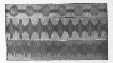
FIGURE 24—Sample Fast Records Showing Distortion Produced by Intentional Frequency Modulation. *a* Day Record, *b* and *c* Night Records
