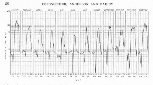
Monthly Averages of Diurnal Variation of Signal Field Strength. Rocky Point, L. I., U. S. A. (2XS) Measured at New Southgate, England. Cor-rected to 300 Amperes Antenna Current 5,480 Km.
