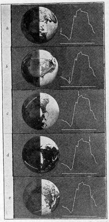
FIGURE 7—Diurnal Variation in January Signal Field. a. Total Path in Sunlight. b. Sunset Near Midpoint of Transmission Path. c. Sunset Conditions When High Night Values Have Been Obtained. d. Sunrise Conditions When High Night Values Begin to Decrease. e. Sunrise Near Midpoint of Transmission Path
