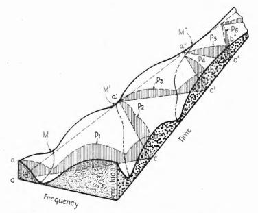
FIGURE 18—Three Dimensional Diagram, Showing the Method of Interpreting Band Fading Records
