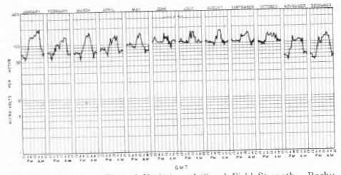
Monthly Averages of Diurnal Variation of Signal Field Strength. Rocky Point, L. I., U. S. A. (WQL) Measured at New Southgate, England. Corrected to 600 Amperes Antenna Current 5,480 Km. 17,130 Cycles
