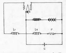
FIGURE 45—Diagram of an Oscillator Circuit
