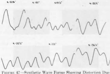
FIGURE 47—Synthetic Wave Forms Showing Distortion Due to Frequency Modulation
