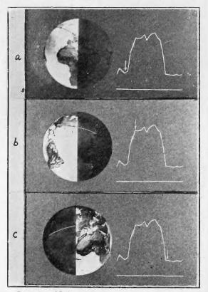
FIGURE 19—January Noise. a. Sunset Conditions as Night-time Noise Begins to Increase. b. Sunset Conditions When Noise Has Reached High Night-time Values. c. Sunrise Conditions When Noise Has Reached Normal Low Values
