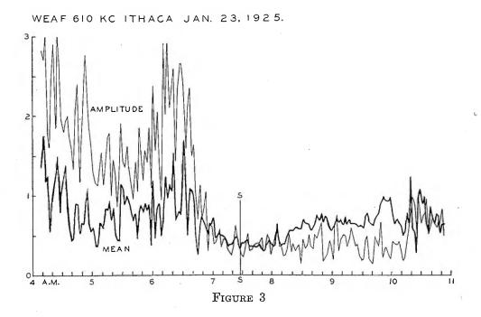
The entire morning record, of which Figure 2 is a portion, is replotted in Figure 3. The vertical line S-S marks sunrise at Ithaca, and, so far as the curve is concerned, apparently determined a "low." About an hour before sunrise there is a marked peak in both curves, and preceding this, about two hours before sunrise there is another low. This is quite a normal beforesunrise performance, which was in fact repeated for this station on the eclipse morning.
