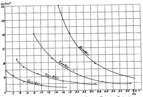
FIGURE 11-Iube DT-1, Experimental Curves, Detector Output
