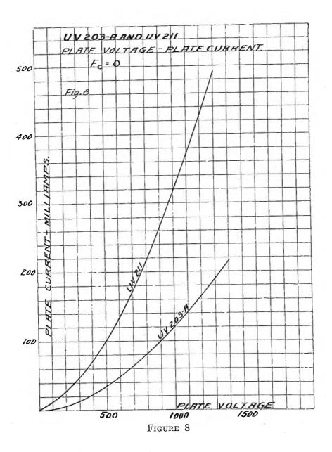
UV-203-A and UV-211 curves plainly indicate the superior characteristics of the X-L filament tubes.
