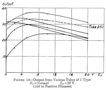
tubes it appears that the one having the 1.1-volt filament happens to approach the required grid bias conditions most closely when connected in this way.
