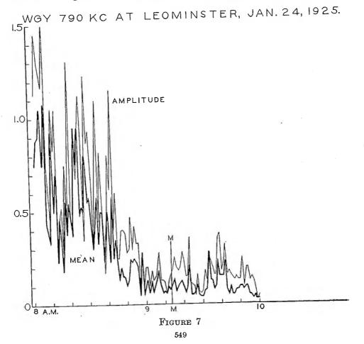
nearly half an hour at the middle of the eclipse, and superposed on this general lowering is a fall before and a rise after the middle which resembles that shown in Figures 4 and 5. But a still more marked fall and rise center on 9.30 A. M., so this record is not by itself conclusive.
