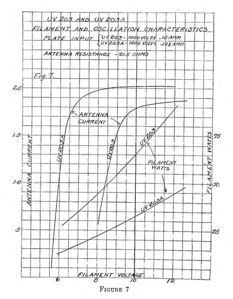
half the filament power and at one-sixth less plate current than is taken by the UV-203. At the normal operating point, the UV-203-A gives over 20 percent greater oscillation efficiency than the UV-203.
