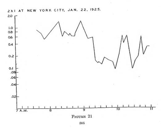
shown, the detector current changing over ten-fold, corresponding to a field decrease of over three times.
