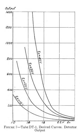
ing of M is the same as it was when no signal was coming in. The amount of additional grid bias necessary to bring about this result, as measured on the voltmeter V, is equal to the peak voltage of the signal in the secondary of the transformer T, and, therefore, proportional to the change in plate current in the detector tube, within reasonable limits of operation.
