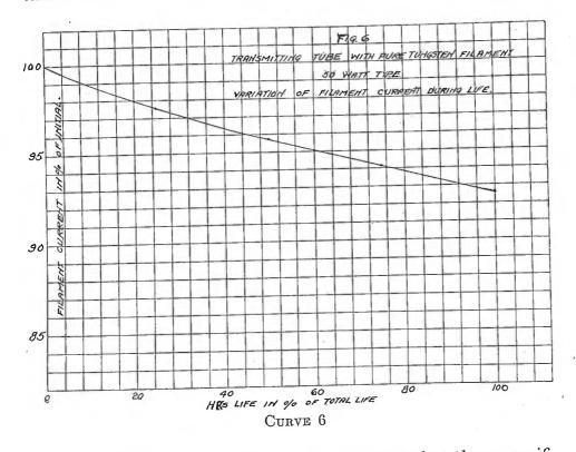
In conclusion, it is again to be emphasized that these specific results have been selected to illustrate some of the results obtained from the life testing of triodes, but by the very nature of the tests and the way triodes are used, they cannot in any way represent the life to be expected in any individual case of operation.
