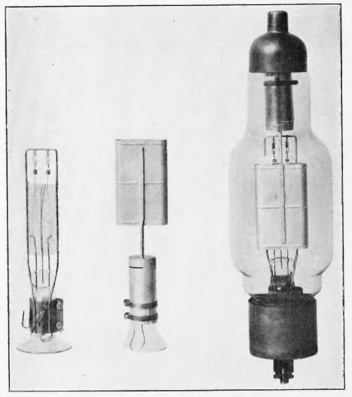
FIGURE 10-Radiotron UV-204-A 250-Watt Output
