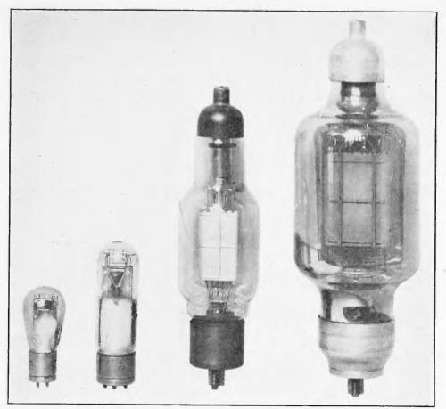
FIGURE 1-X-L Filament Transmitting Tubes
