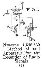
METHOD OF AND APPARATUS FOR THE RECEPTION OF RADIO SIGNALS, by impressing the received signaling energy upon the anode-cathode circuit of a thermionic impedance. The impedance is independently varied by varying an electrostatic field at predetermined frequency different from the incoming signaling frequency whereby the signaling current may be translated into intelligible sounds.
