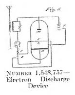
ELECTRON DISCHARGE DEVICE, which includes a cathode and two anodes. A cathode is provided and the circuits arranged so that electrons flow to both of the anodes. The circuit is such that the potential of one of the anodes may be varied with respect to the cathode and the flow of electrons to the anode may be increasingly diverted to the other anodes as the potential of the first named anode is increased. The tube may be used as an amplifier and is termed in the specification "a negatron."
