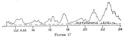
Figure 17, which is a reception record taken in Newton Centre, Massachusetts, from KGO at Oakland, California, shows a fading curve which is very much like that of Chicago stations of similar transmission frequency. This record is also interesting in that it shows a low disturbance level on that particular night; unfortunately this is not normal at my receiving point.
