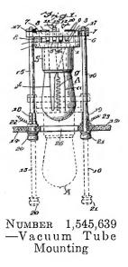
VACUUM TUBE MOUNTING, in which the electron tube is carried upon a movable structure by which the tube may be normally disposed within a cabinet and withdrawn to permit removal or re-insertion of a tube in the socket member. The socket member is guided by rods on opposite sides thereof enabling it to be readily moved to a point adjacent the front of the panel or returned to a position behind the panel when the tube is to be inserted or removed from the socket.
