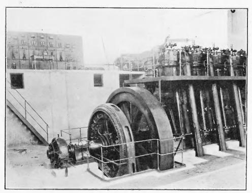
FIGURE 10—Interior of Power House Showing Diesel Engine and Steam Turbine and Switchboard in the Balcony in Background
