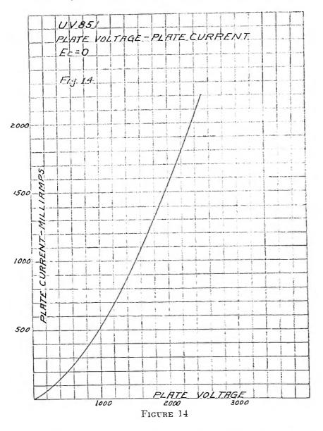
acteristics required to give one-kilowatt output with reasonable efficiency at the relatively low plate voltage of 2,000 volts would have been unattainable with a tungsten filament.
