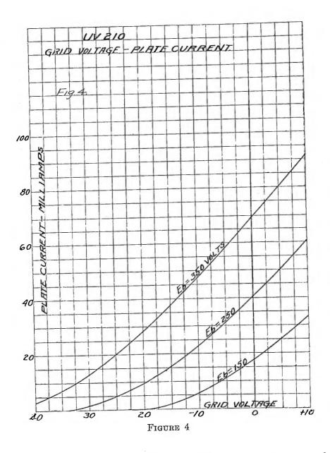
In addition to its use in transmitting sets as oscillator, modulator or power amplifier, this tube has been used to some extent in commercial receiving circuits where the service is continuous and where the power output is unusually high, requiring plate voltage and plate current conditions nearly as severe as in transmitting circuits.
