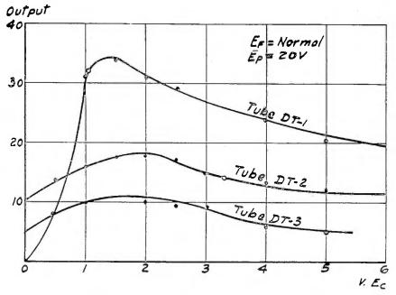
FIGURE 13-Variation of Detector Output with Grid Voltage
