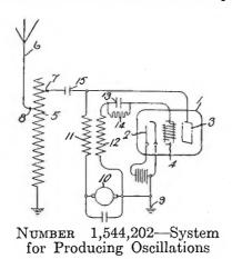
SYSTEM FOR PRODUCING OSCILLATIONS by use of an electron tube which has an oscillating circuit coupled to a shunt circuit between its cathode and anode. The input and output circuits of the tube are coupled, but the frequency of the oscillations is determined principally by the constants of the oscillating circuit. 1,544,486-J. Sedlak, filed May 31, 1924, issued June 30, 1925.
