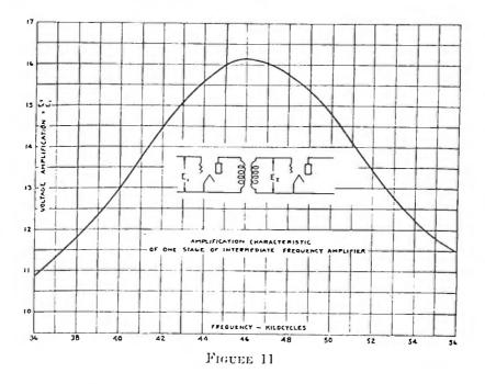
MEASUREMENT OF THE INTERMEDIATE FREQUENCY AMPLIFIER
