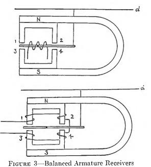
The chief advantage of a strong field in this type of receiver is that the sensitivity is greater. The double frequency component of force, so objectionable in the simple receiver, is not present in this type if the armature is closely balanced. That there is no double frequency pull may be shown as follows: The pull caused by poles 1 and 4 is proportional to
