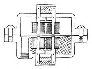
FIGURE 5—Balanced Diaphragm Receiver
