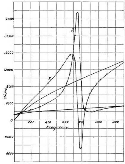
FIGURE S-Resistance and Reactance Curves
