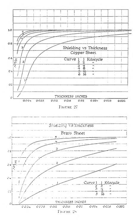
The shielding depends on the resistivity of the shielding metal for a definite frequency and thickness as shown by the curves of Figure 33.
