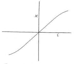
FIGURE 4—Static Characteristic of Balanced Receiver
