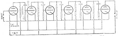
FIGURE 3-Six-Stage Resistance Condenser Coupled Amplifier
