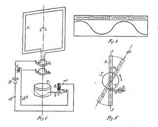
NUMBER 1,525,177—Direct Reading Radiotele graphic Compass
