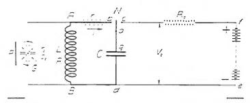
Frotune 4—Schematic Representation of the Arrangement. The test-circuit is shown in heavy lines, G is a Quadrant-Electrometer connected up as shown and resting on a grounded plate P (see also Figure 5). The one terminal e of the battery is also grounded.
