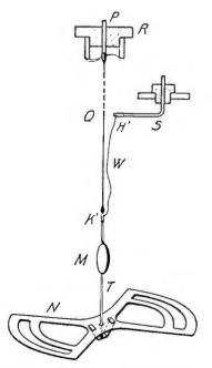
FIGURE 7—New Method for suspension of the needle and for providing electrical connection. (Compare Figure 5a.) In the tests described below, the quadrant electrometer had a quarts wire 90 mm. in length and 0.01 mm. thick. The Wollaston wire was about 50 mm. long and 0.004 mm. thick. The needle was made of aluminum foil 0.02 mm. thick.
