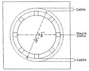
FIGURE 17-Section Thru Control Coil Support
