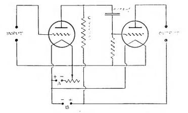
FIGURE 4-Resistance Coupled Amplifier for Zero Peat Indicator
