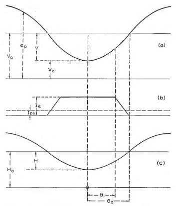
FIGURE 18—Plate Voltage, Plate Current and Magnetic Field Relationships in Magnetron Oscillator
