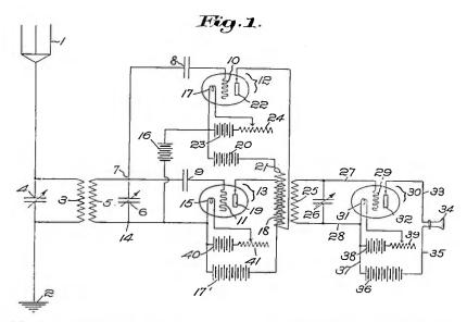
NUMBER 1,526,852—Means for and Method of Limiting Interference in Radio Signaling
