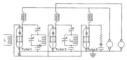
FIGURE 9-Circuit for Determination of Amplification per Tube
