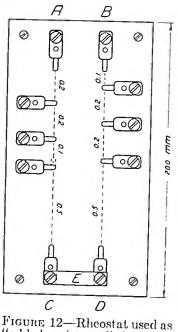
"added resistance" in these measurements and made of a single 0.3 mm. Constantan Wire
