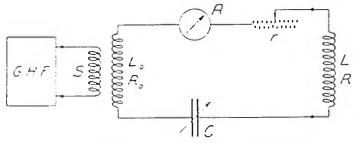
FIGURE 2-The Added-Resistance Method
