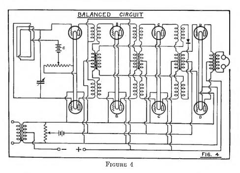
This circuit includes 8 De Forest DV-2 amplifier tubes, one crystal detector, 6 radio frequency transformers, 4 audio frequency transformers, 3 step-up transformers, and one step-down transformer. The step-down transformer was the output transformer for the telephones. The three input transformers were balanced type. The "B" battery supply is rectified alternating current, but the filaments were lit with alternating current. Power was delivered from a six-volt step-down transformer.
