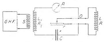
FIGURE 1-The Substitution Method
