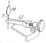
FIGURE 5b—Details of clamping arrangement. The tweezerform spring U is made of phosphor-bronze and is opened and closed by means of a conicalpointed screw in such a way that on closing, the wire T with needle and mirror is raised a little by the spring
