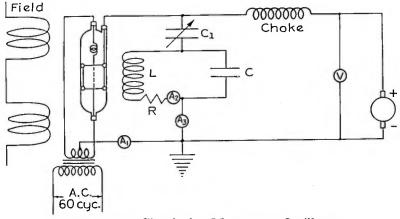
FIGURE 15—Circuit for Magnetron Oscillator
