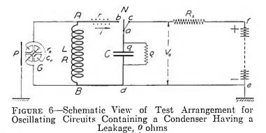
Here the terminals a and c are connected together so that the terminals of the condenser C having a leakage of q ohms are permanently connected to the terminals e and f of the battery. The discharge is then started immediately when the contact ab is made, and at the beginning of the discharge the condenser has the charge  $V_oC$ —assuming that  $q \gg R_o$ , where  $R_o$  is a large resistance inserted in the lead  $c f.^7$
