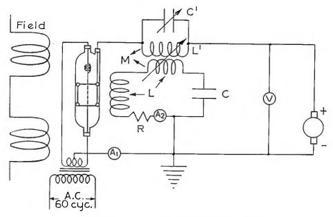
FIGURE 14—Circuit for Magnetron Oscillator
