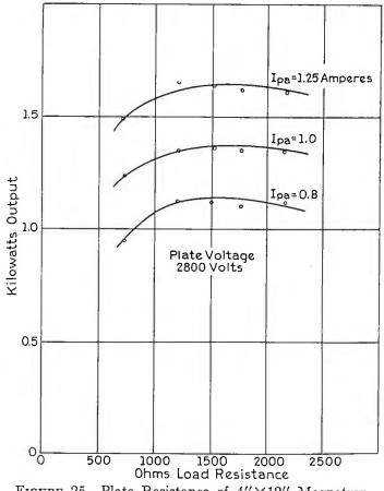
FIGURE 25—Plate Resistance of 4"×12" Magnetron
