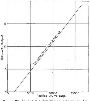
FIGURE 23—Output as a Function of Plate Voltage for  $4'' \times 12''$  Magnetron
