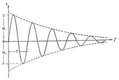
FIGURE 3—Curve of Oscillations
