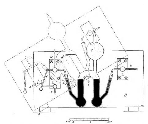
FIGURE 8—Key I. Mercury lamp used as discharging key. The connecting wires a, b, and c. corresponds to the connections denoted by the same letters in Figures 4 and 6. Using the arrangement of Figure 6, a and c are directly connected, thus shunting out the interrupter f. This is also the case with the keys shown in Figures 9-11.  $E_1$  and  $E_2$  are ebonite pieces. Similar lettering is used in Figures 9-11
