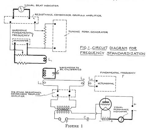
two frequencies are very different, but such a shift of frequency is not likely to happen during the measurement and after having the fundamental frequency f adjusted. The visual indicator of resonance will indicate a sharp minimum whenever the wavemeter is tuned to the fundamental frequency f or any integral multiple of it. The procedure of measurement is briefly as follows:
