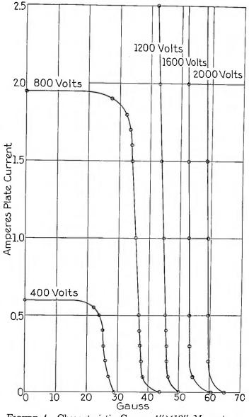
FIGURE 4—Characteristic Curves 4"×12" Magnetron
