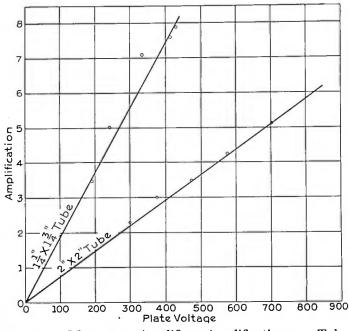
FIGURE 10-Magnetron Amplifier-Amplification per Tube
