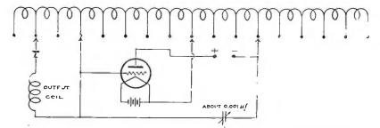
FIGURE 2-Diagram of Connections for the Harmonic Generator
