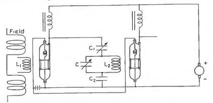
FIGURE 5-Circuit for Magnetron Amplifier
