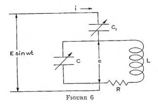
current *i* will flow thru the circuit and a voltage *e* will be set up across *C* and *L*. As is usually the case with radio circuits, the resistance of the coil *L* can be neglected in comparison with  $\omega L$ , and thus in the complex notation,
