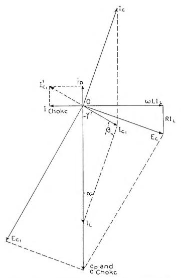
FIGURE 24--Vector Diagram for Magnetron Oscillator
