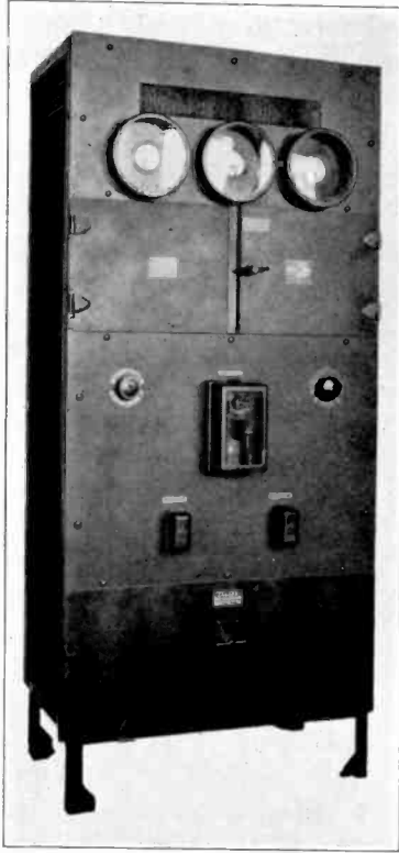
FIGURE 7—1 Kilowatt Broadcasting Radio Telephone Transmitter
