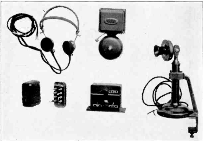
FIGURE 5—Extension Station Equipment for Radio Telephone Transmitter
