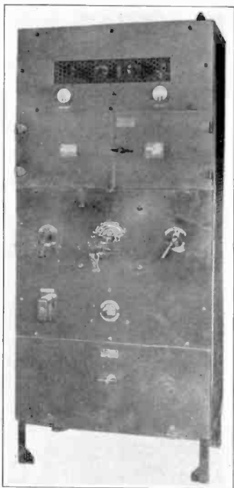
FIGURE 1—1 Kilowatt Commercial Radio Telephone Transmitter
