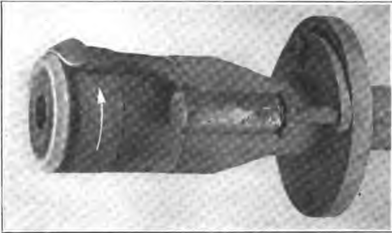
FIGURES 4A and 4B—Cathode with a Cooling Shoe. a inlet, a' outlet for water. The cathode proper is rotated as indicated by an arrow
