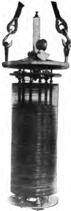
FIGURE 7—Compressed Air Condenser
