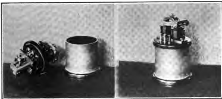
FIGURE 4—Oil Break Relay Key
