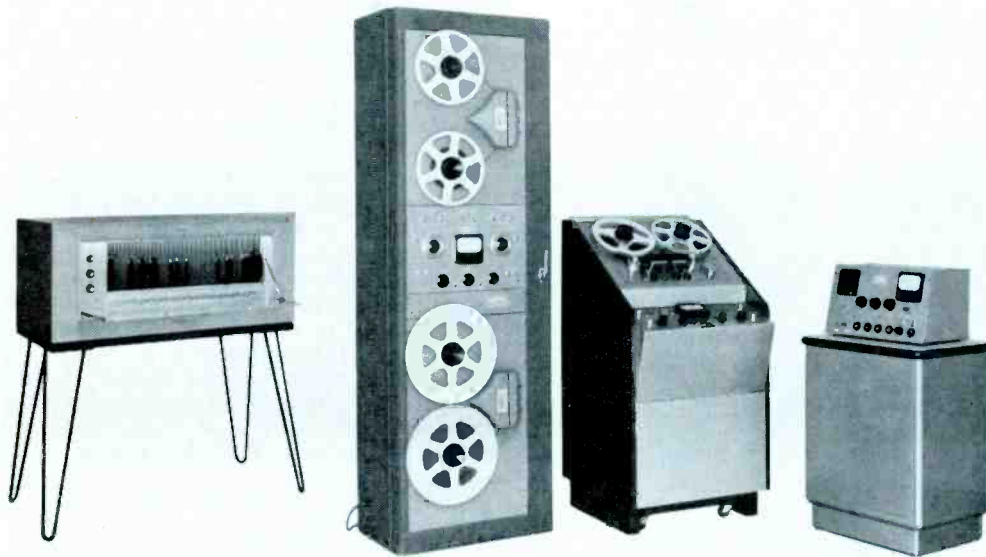
Fig. 3 - The Ampex S-3380 Automatic Program System and Seeberg record changer. The rack mounted equipment includes a 7 1/2 ips announce tape reproducer, the automatic control unit, an optional panel for controlling an automatic record changer, and a 3 3/4 ips program tape reproducer. This system includes a master timer for automatically reproducing the station identification on the hour and half hour as well as an electronic fade system which fades the music when announcements and music overlap.
