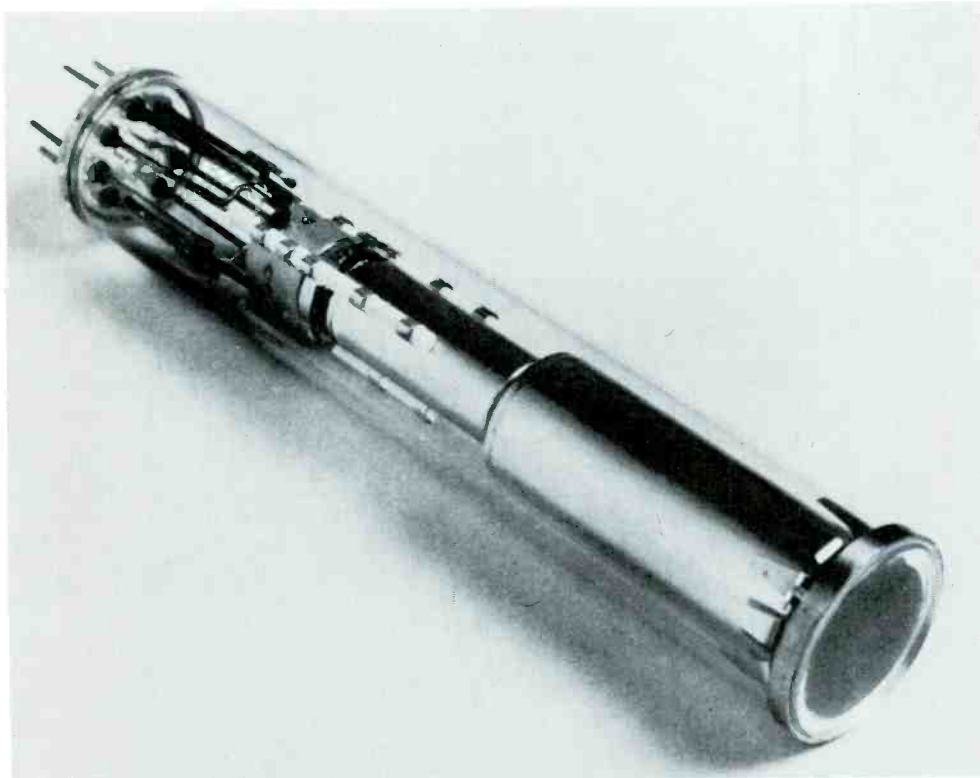
Fig. 15 - Photograph of improved developmental vidicon.
