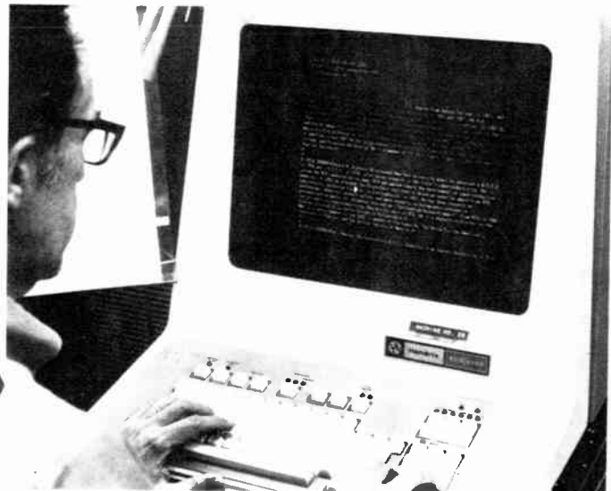
CRT editing terminal. Using the Hendrix 5200 terminal, a skilled operator inserts corrections into the stored data. Complex specifications covering type style (font), size, and spacing (leading, measure) are given as simple “macro” codes. For each such code, the 2050A computer produces specifications for driving the phototypesetter.
