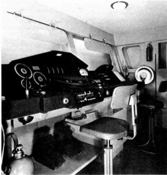
[5] Driver's cabin in a class CC 72000 diesel-electric. Directly in front of the operator (whose position is in the left center of the cab) is a massive console, containing from top to bottom: two ammeters for each of the two electric traction motors; one motor per bogie and two voltmeters; a signaling board for auxiliary devices and wheel slippage. The large circular dials to the left are the diesel tachometers; the white dial on the right is the speedometer/odometer. In all, the dials are very well positioned.
