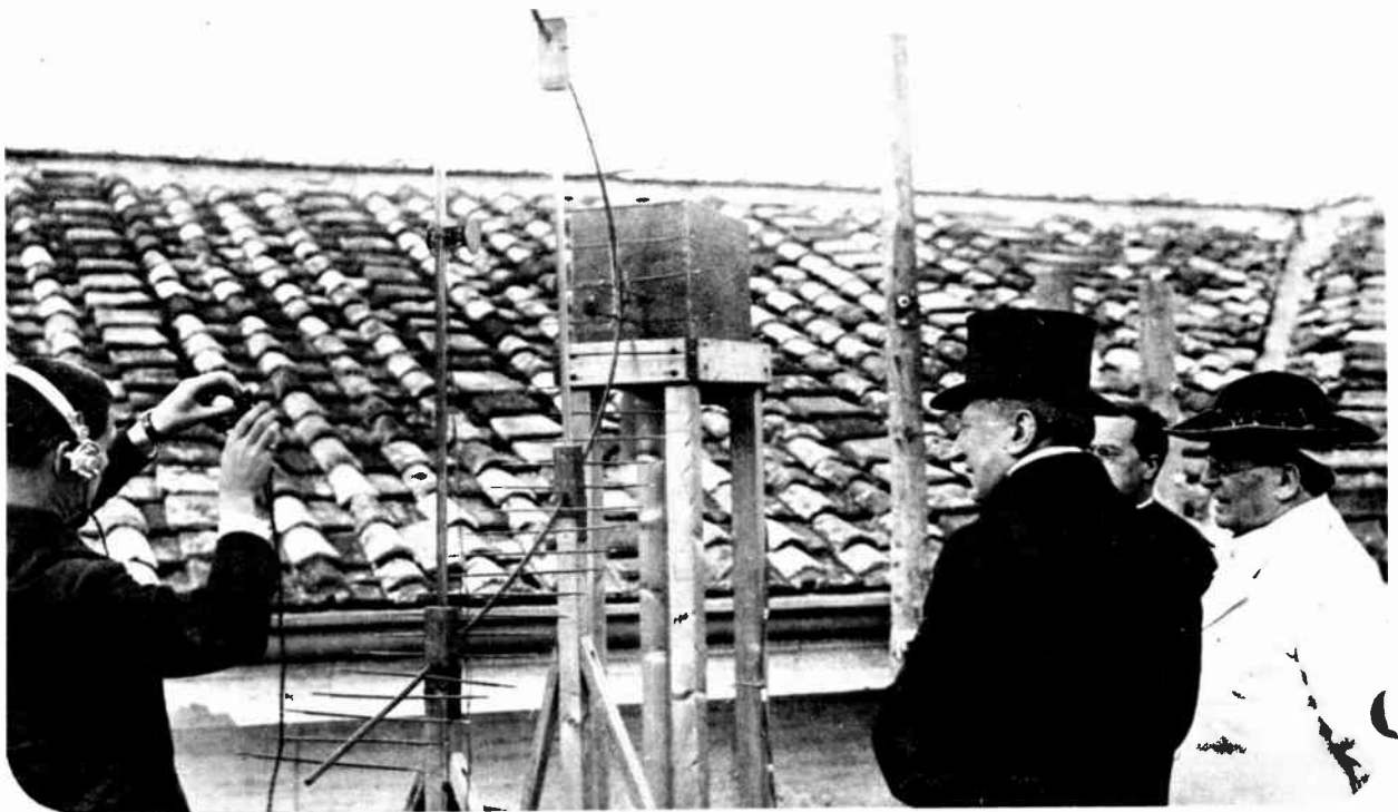
A pioneer ultrashort-wave radio circuit was established between the Vatican and the Pope’s summer residence, Castel Gandolfo, in 1933. Marconi, to the right of the directive antenna, is shown with Pius XI.
