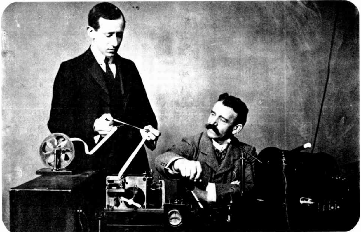
Guglielmo Marconi (left) and George Kemp. A photograph taken shortly after the successful transatlantic test of 1901. The 10-inch induction coil spark transmitter is on the right, with Morse inker and 'grasshopper' key in center.
