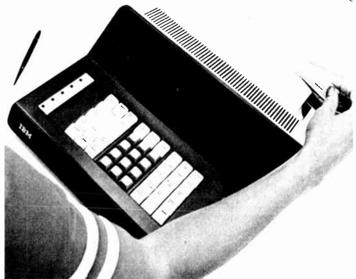
[2] Slot-type reader on top of IBM 3604 keyboard display terminal for finance applications can read magnetic-stripe or identification cards, as well as passbooks.
