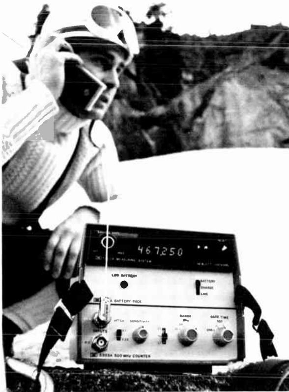
Mobile transmitters, restricted to precise frequency assignments, can be quickly field-tested with Hewlett-Packard's 5300 series measurement system. As illustrated above, the mainframe, battery pack, and functional module snap together to form a 500-MHz counter.
