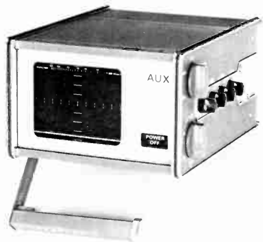
[1] The Tektronix 410 physiological monitor.
