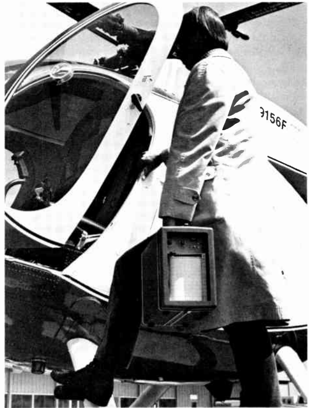
Portable strip chart recorders work on location while preserving data for later comparison and analysis. This Hewlett-Packard model 7155A has 0.1-mV to 10-volt per division input sensitivity, and disposable pens, which eliminate ink loading problems. Price for the basic unit is $985.
