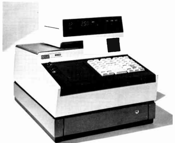
[4] Intelligent cash registers with built-in microcomputers are finding widespread application in retail trade. This supermarket register contains a microprocessor with both core, and read-only MOS memories.
