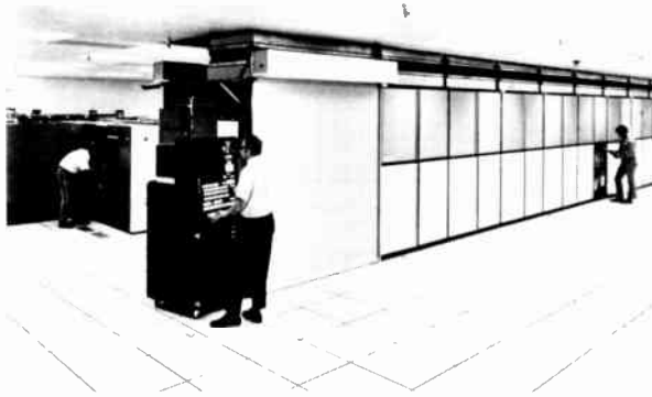
[2] This floor-full of equipment is the Illiac IV supercomputer, recently installed at NASA's Ames Research Center. The giant machine not only services local computation needs, but is connected—via the ARPA network—to many computers and terminals in other locations.
