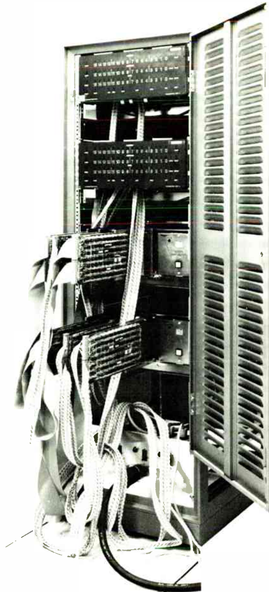
[2] Packet communications will be speeded by this Interface Message Processor (IMP) designed for operation with 1.3-Mb/s links.
