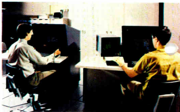
TYPICAL interactive graphic IC layout at Texas Instruments uses two large interactive screens and a small storage screen. The large screen on the left shows the circuit schematic; the large screen on the right displays the area of the IC now being designed. The small screen shows a composite layout.
