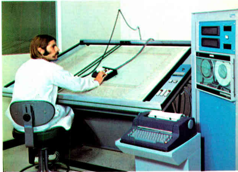
THE CALMA COMPANY'S 485 system (below), part of a semiconductor photomask artwork generation system at Micro-Mask. In addition to the digitizer shown, the system includes an off-line CalComp flatbed plotter.
