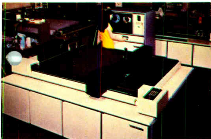
CALCOMP'S 745 flatbed plotter and model 900 controller is shown above. The model 745—with a drafting surface of polished granite and a recirculating-ball lead-screw drive system—uses model 900 software to cut rubylith, expose photographic film, or make multiple-line-width drawings.
