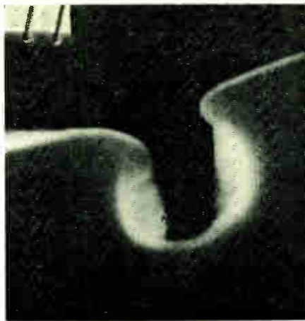
FIGURE 7. Electron-beam spreading in resist material creates an exposed volume much larger than the beam diameter, as shown here. An electron beam was scanned across a thick resist, as shown, to create the cylindrical volume.
