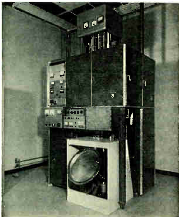
FIGURE 16. Ion implantation system for carrying out the implantation step in the manufacture of MOSFET integrated circuits. The terminal housing, including ion source, is shown at the top and the rotating multiple-target chamber at bottom right. (Figures 15 and 16 courtesy Hughes Aircraft Co.)
