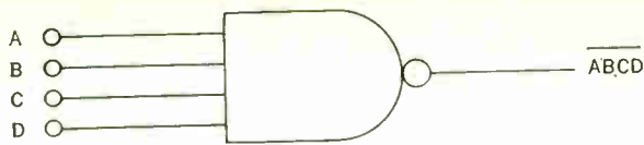
FIGURE 35. TTL basic gate, which performs the NAND logic function. The “implied AND” connection is not possible because of the “active pull-up.”
