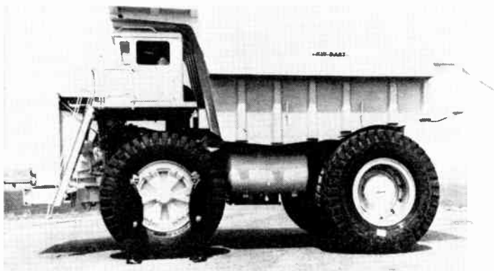
FIGURE 4. 150-tonne diesel-electric truck driven by two "motorized" rear wheels.
