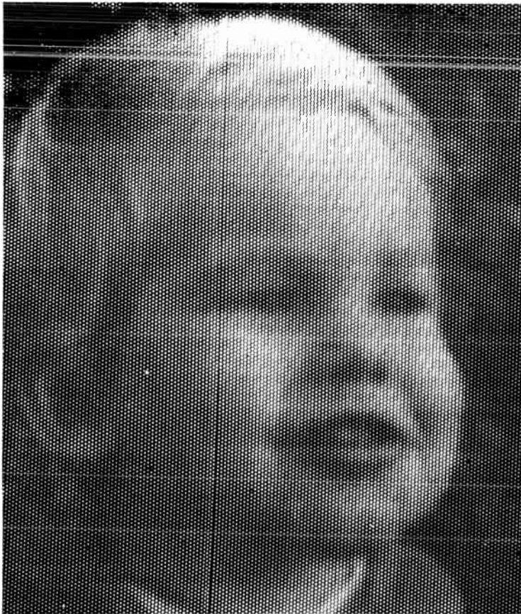
FIGURE 3. Hex-format white-dot structure—110-line screening in original; this reproduction magnified approximately 3.15X for clarity in illustrating the hex structure.
