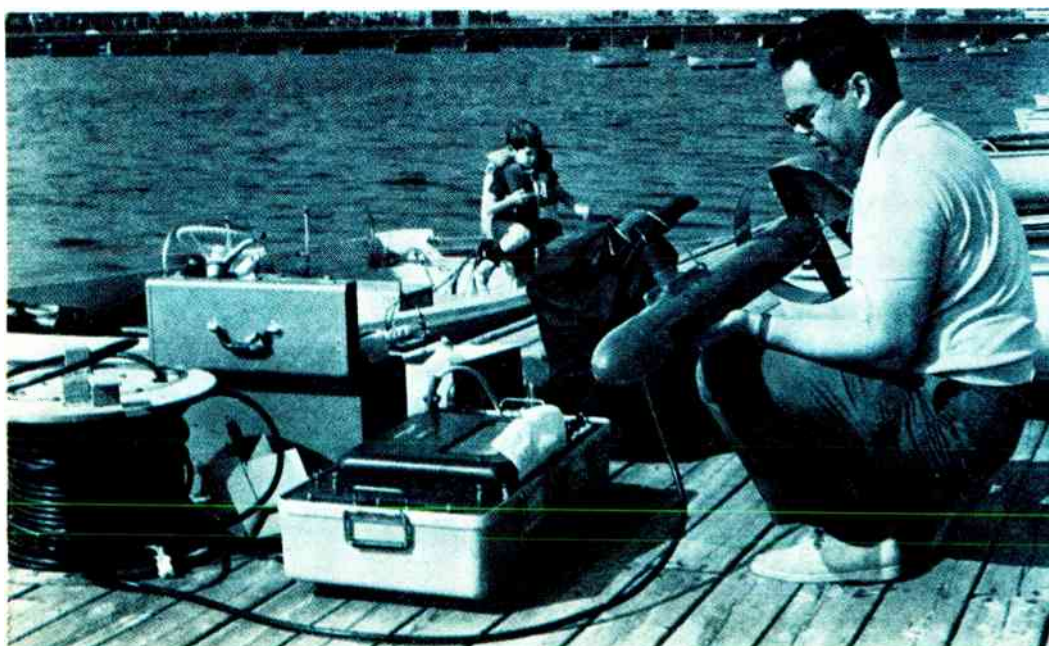
FIGURE 1. Battery-operated dual-channel portable 200-kHz side-scan system. Robert Henderson of EG&G International, Inc., is holding the towfish. The entire system can be used from the Boston Whaler shown at the M.I.T. sailing pavilion.
