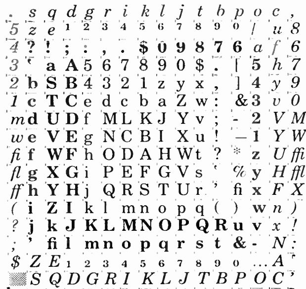
FIGURE 9. Typical Linotron character grid, containing 256 alphanumeric characters and standard symbols in roman, italics, and bold face.
