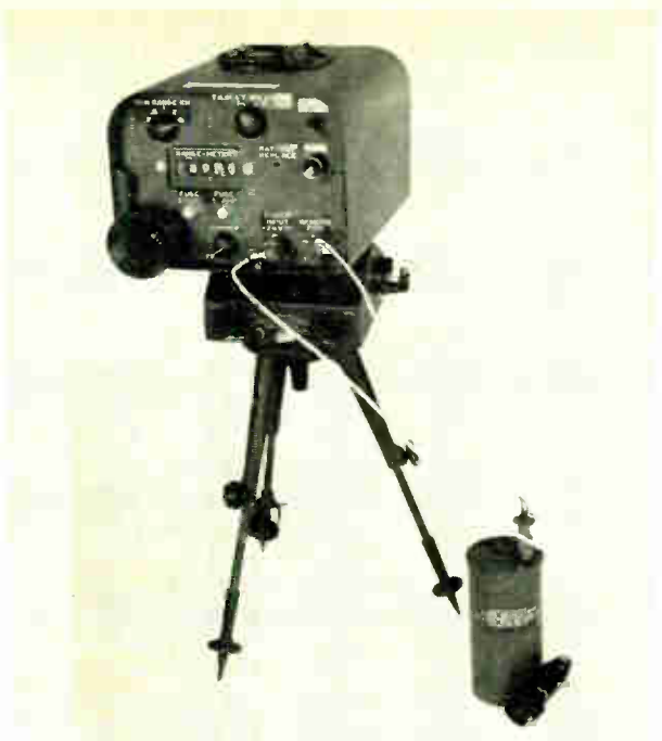
FIGURE 5. Example of a laser range finder, representing one of the most advanced of all laser devices. Range is determined by a time-of-flight measurement of a pulse and its reflection. The data are displayed in digital form.
