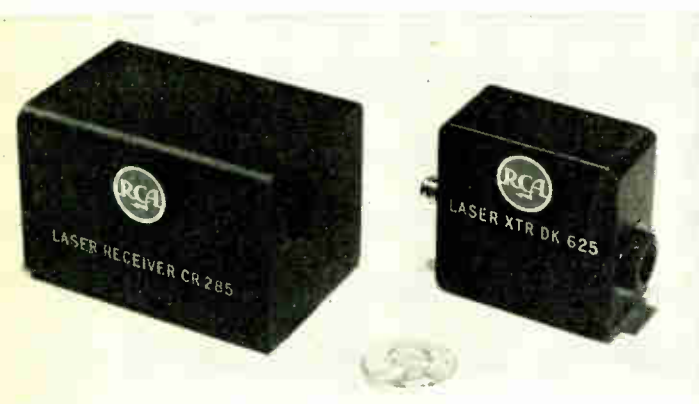
FIGURE 7. Laser intrusion alarm employing an 8-watt diode. A 300-volt battery produces a 200-pulse-per-second 70-ns output. With only modest effort the transmitted pulses can be coded to render the system "spoof-proof." When used with appropriately positioned reflectors, the transmitter and receiver can be placed side by side in a region safe from the local environment.
