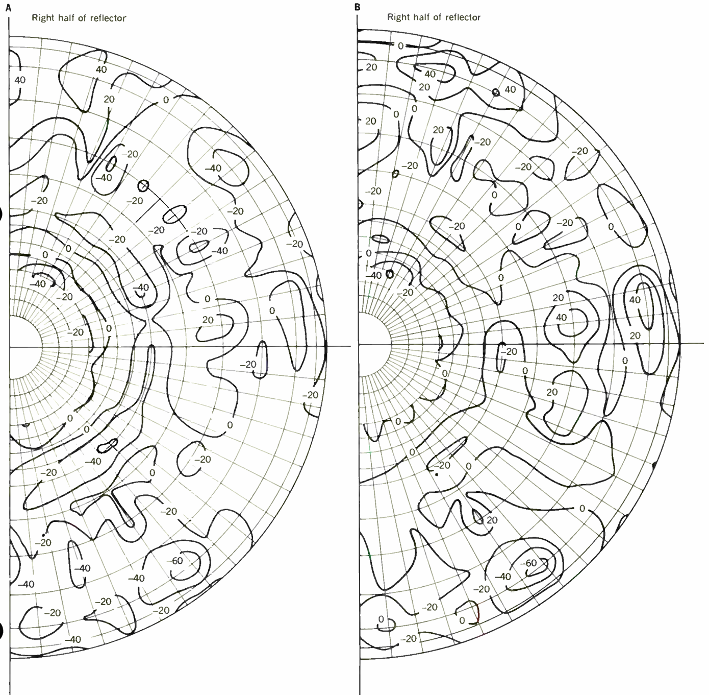
Fig. 9. Peak deviations of reflector surface, as rigged May 14, 1964, calculated from face-up survey data plus calculated gravity effects (nominal temperature environment). Numbers represent peak departures from an ideal parabolic contour in thousandths of an inch. A—30° elevation angle. B—60° elevation angle.
