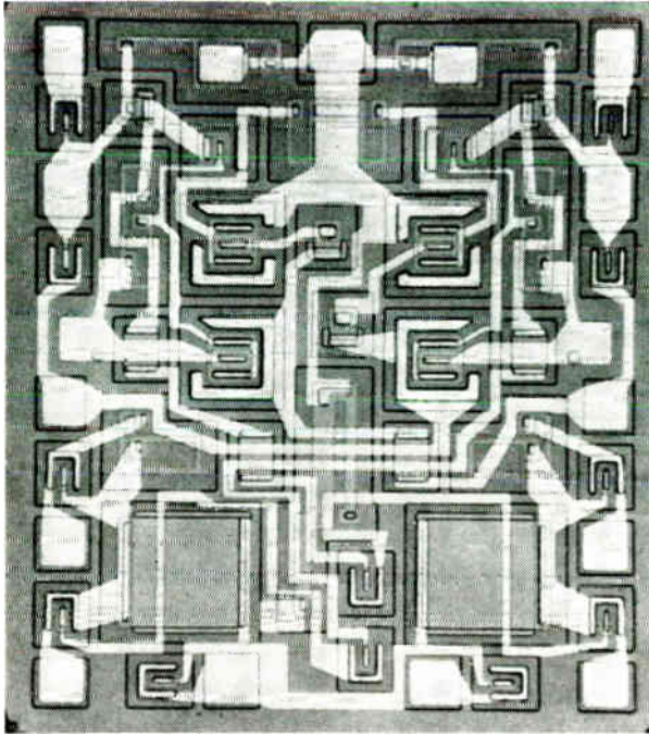
Fig. 18. The current level of practical complexity is illustrated by this gated flip-flop or pulse binary. It contains 45 components with about 12 to 14 leads. The resistors and capacitors are diffused; the transistors are n-p-n units.
