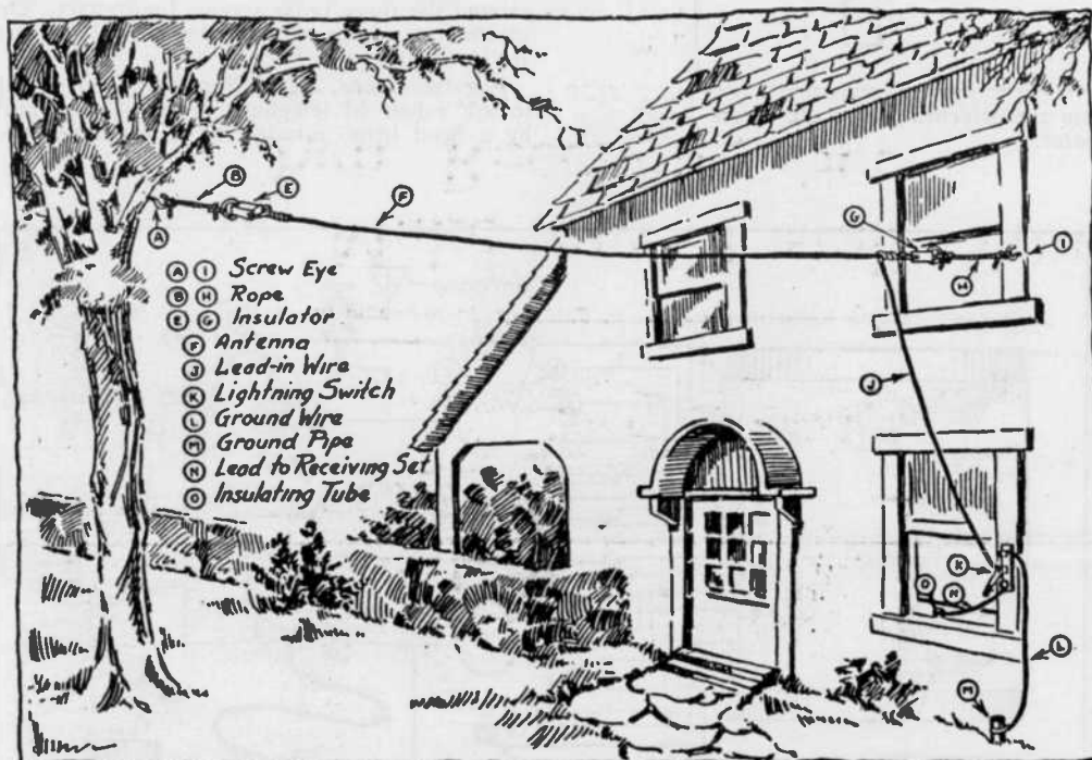
FIGURE 1; A simple arrangement of stringing the antenna between a house and tree.
