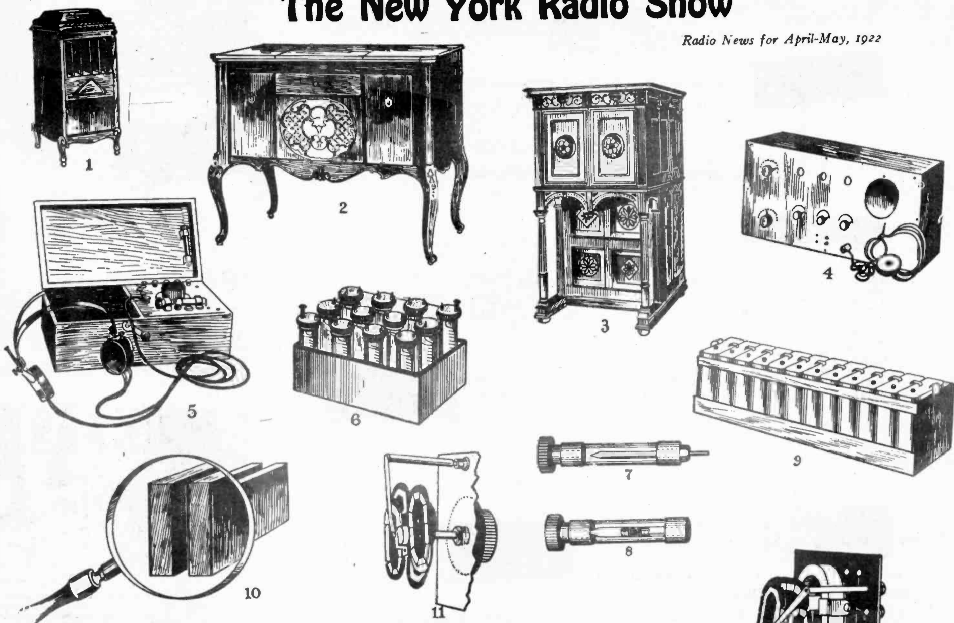
Figs. 1, 2 and 3 illustrate new types of receiving cabinets exhibited to the public for the first time at the Radio Show. Everything necessary for the reception and reproduction in loud tones of radiophone transmission is included in the handsome cabinet. Controls are greatly simplified. Figs. 2 and 3 also include a phonograph using the same loud speaker as the radio receiver, and Fig. 3 employs an electric blower to increase the sound. Fig. 4 is a simple and complete receiving set intended for the novice in radio. There are only two controls in addition to the filament rheostat. Loud speaker is built in the same cabinet. Fig. 5 is a complete and very compact receiver employing vacuum tube of recent design which requires no plate battery. Everything except the antenna is included in this small cabinet for the reception of the signals, and wave lengths ranging from 100 to 1,000 meters are obtained by single control. Fig. 7 is the vacuum tube used in this receiver and Fig. 12 is a back view of the same receiver removed from the cabinet. The fixed magnet seen in Fig. 12 acts upon the flow of electrons in the tube and aids detection. The variometer, which is clearly shown in Fig. 11, is of unusual design and very compact. Figs. 6 and 9 illustrate two new types of storage plate batteries. These may be recharged. Fig. 8 is a crystal detector enclosed in a vacuum to prevent oxidation. Fig. 10 shows two kinds of panels, one with copper shielding inside the panel for prevention of body capacity effects and the other is made of fibre with bakelite veneer to reduce the cost.
