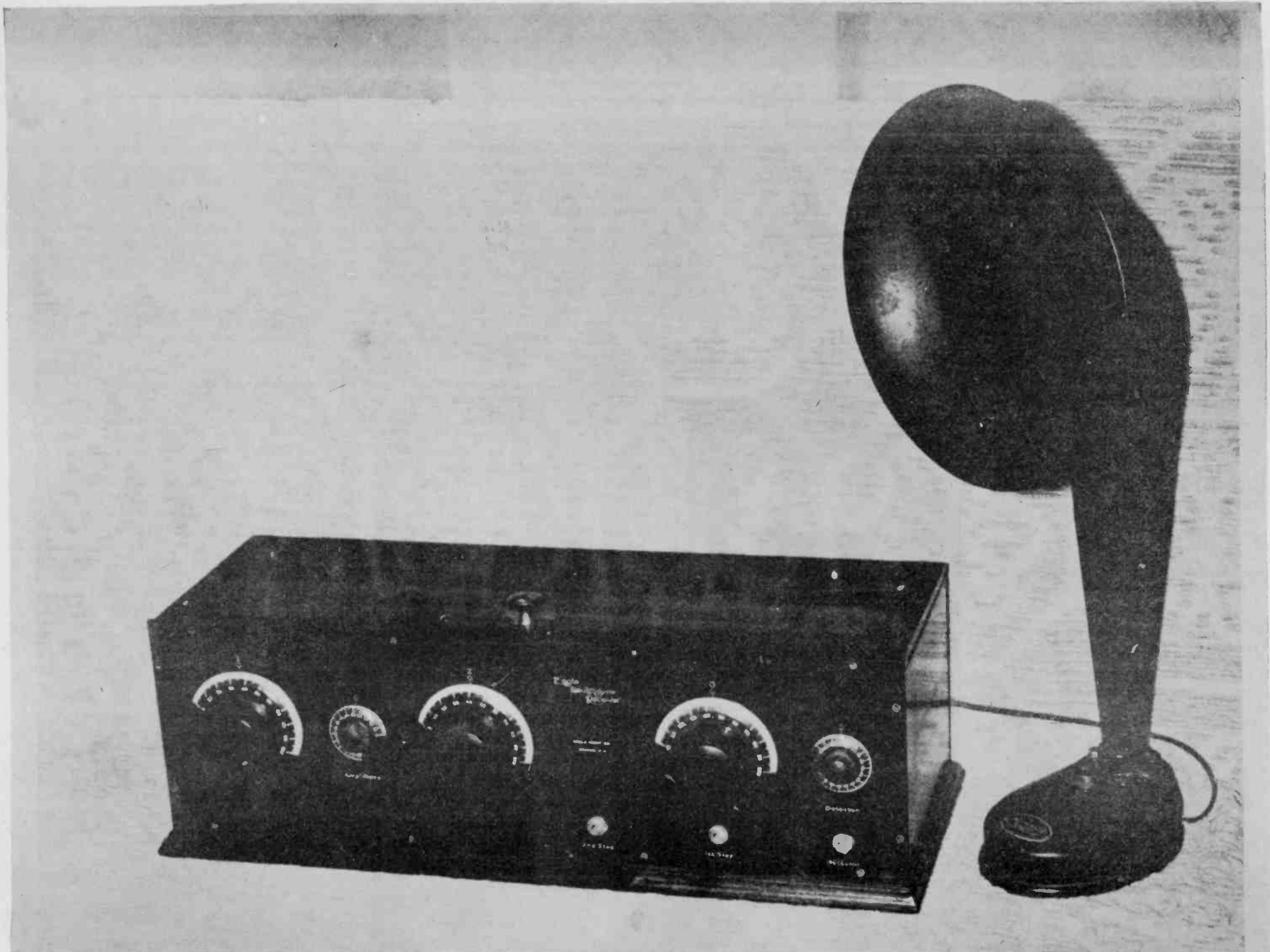
A good looking pair, the Eagle Neutrodyne Receiver and a Dictogrand horn speaker. The Eagle was called a balanced receiver in 1923 when it was sold for $135.00. Now, many collectors are paying the same price.
