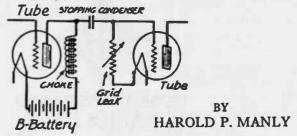
Fig. 1.—The Impedance Coupled Audio Amplifier.
