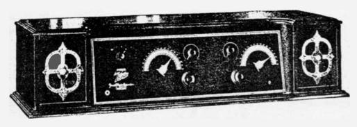
Super-Zenith VII (Not regenerative)—6 tubes—2 stages tuned frequency amplification—detector and 3 stages audio frequency amplification. Installed in a beautifully finished cabinet of solid mahogany—4% inches long, 16% inches wide, 10% inches high. or panels inlaid. Slanting panel of sheet bronse, mahogany finish, with scales and indicators in metallic relief. Gold plated pointers, to prevent tarnish. Compartments at either end for dry batteries.
