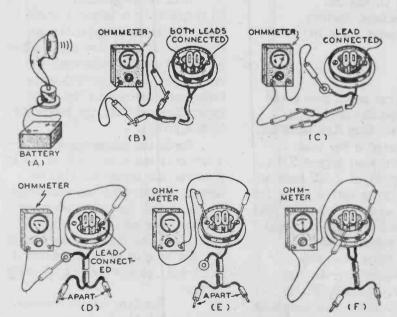
FIG. 26-8.—Various electrical tests which should be made on a magnetic loud speaker of either the *iron-diaphragm* or balanced armature type in order to locate electrical trouble in either the speaker cord or the coils.
