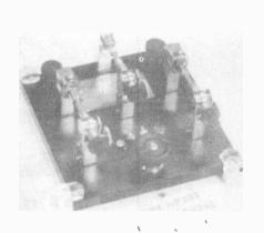
A type I-P 203 triple crystal detector by Wireless Specialty Apparatus Co. One of Leo Rayner's rare items.
