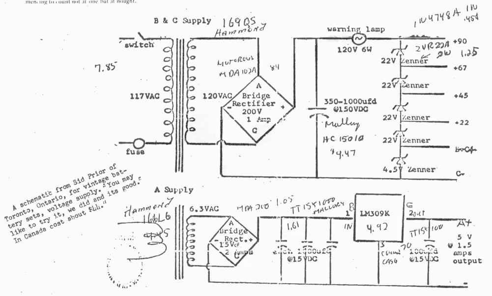
Radio Shack offers a printed circut board for the 5V A Supply and all of the parts needed for it. The transformer for the B-C Supply can be a constant voltage transformer or 115 to 125 VAC out. The bigger the capacitor in the B-C Supply the better, but they are expensive (36 to \$8). The Zenners are very cheap from Solid State Sales, P.O. Box 74D, Somerville, Mass. 02143.
