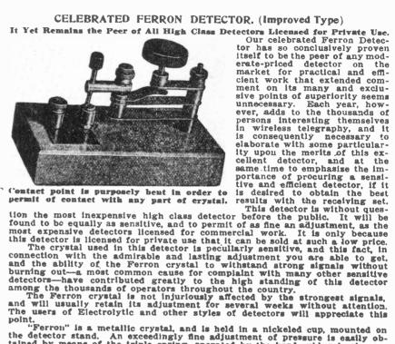
and will usually retain its adjustment for several weeks without attention. The users of Electrolytic and other styles of detectors will appreciate this point.
