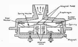
Fig. 26-9. — Crossical horn-type irondiaphragm loud speaker unit, showing the relative arrangement of its parts. A disassembled unit of this kind is illustrated in Fig. 26-10.
