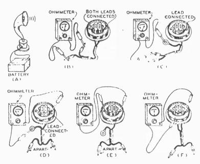
Fig. 26-8.—Various electrical tests which should be made on a magnetic loud speaker of either the iron-diaphragm or balanced arm ature type in order to locate electrical trouble in either the speaker cord or the coils. These tests are described in detail in the accom-
