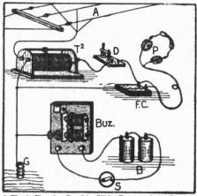
A Hook-Up of a Double Side Tuning Coil, Crystal Detector, Fixed Condensor and Phones, is Shown Above. The Method of Connecting a Buzzer for Testing Crystal Detector is Also Illustrated. A-Aerial, T-Two Side Tuner, D-Detector, F. C.-Fixed Condenser, P-Phones, Buz-Buzzer, G-Ground, B-Battery, S-Switch.
