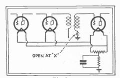
Fig. 3 In an old-fashioned, low-voltage receiver, an isolated grid would block. Now, as Mr. Chambers finds, the tube runs a high plate current.
