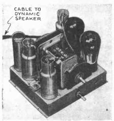
Chassis view of the Model 148 Crosley Book Case receiver. The circuit of this set is different from that shown for the model in Fig. A, above and Fig. I. A description of this receiver appears in the text.
