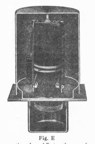
Cross-section of an I.F. transformer; observe "sub-panel" position of shielded R.F. choke.
