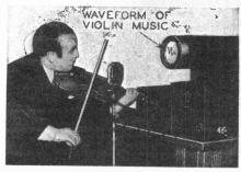
The application of the cathode-ray oscilloscope to waveform analysis in recording.
