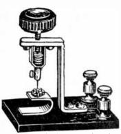
Crystal detector. When the hard rubber knob at the top of the detector stand is turned, the needle point, which presses into the crystal is moved up or down. This allows of a variable adjustment which may be tight or loose, as desired. The spring shown helps to push the crystal up against the needle point.
