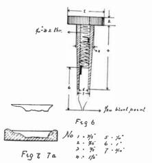
as shown. The point must slide freely in the tube so that when the set screw clamps the tube there will be a constant pressure from the spring, thus holding the point on the Silicon at the same pressure all the time.
