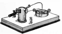
Detector Holder for Galena and Silicon Crystals.
