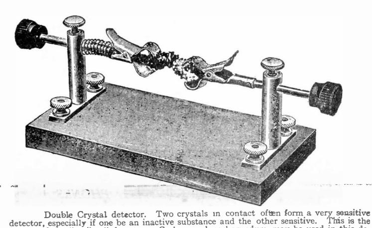
feature of the "perikon" detector. Carbon and carborundum may be used in this de-
